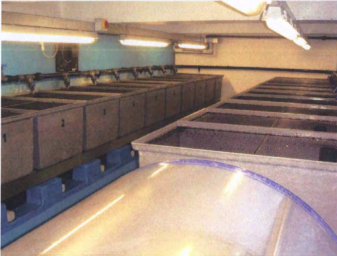
Plate 6.1. Recirculation system (E) based in the experimental aquarium at the University of Plymouth, UK, where the experiment was carried out. The system comprised 20, 125 litre tanks with a flow rate through the tanks of \sim 5 \text{ lmin}^{-1} .
