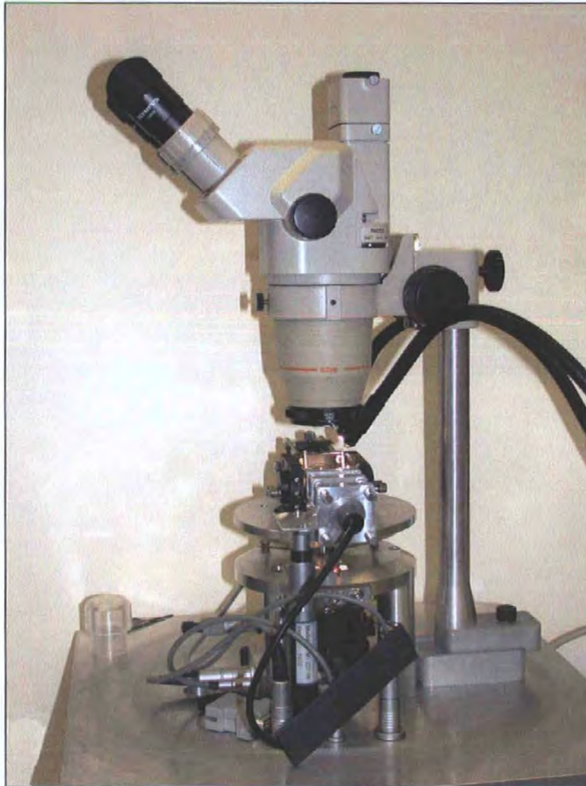
Figure 23. Zoom Stereo Microscope above MFM head.
