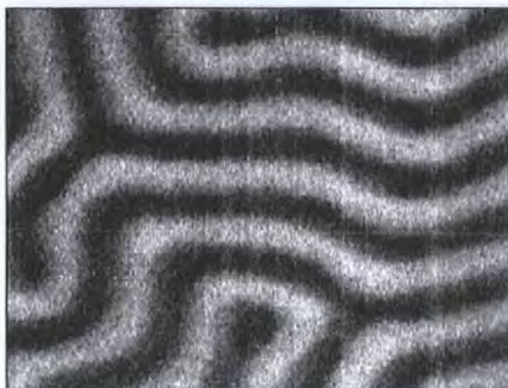
Figure 56. Kerr Effect image of Garnet Layer on Bubble Memory (30 x 40 \mu\text{m} ).
