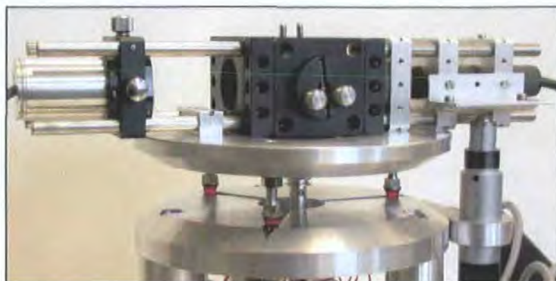
Figure 15. Optical head showing ruby tooling balls for alignment, and DC Motor to bottom right.
