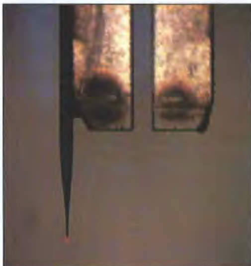
Figure 2. SNOM Probe mounted on tuning fork for Shear-Force control.
