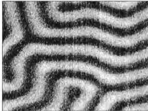
Fig. 3 An image of perpendicular magnetic domain patterns on a bubble memory chip (40mm x 32mm).
