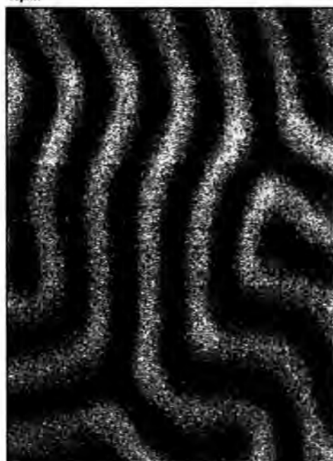
Plate 2 Bubble memory magnetic domain patterns using Kerr effect static laser XY table scan 32\mu\text{m} \times 40\mu\text{m}
