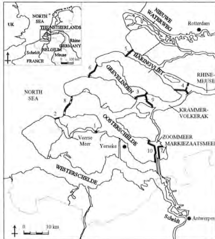
Fig. 1.2. Map of the delta area of the rivers Rhine, Meuse and Scheldt in the SW Netherlands (after Nienhuis and Smaal, 1994). Numbers refer to dam components of the Delta Plan (year of completion in brackets): 1 = Zandreekdam (1960); 2 = Veersegatdam (1961); 3 = Grevelingendam (1964); 4 = Volkerakdam (1969); 5 = Haringvlietdam (1970); 6 = Brouwersdam (1971); 7 = Markiezaatsdam (1983); 8 = Oosterschelde Storm Surge Barrier (1986); 9 = Philipsdam, (1987); and 10 = Oosterdam (1986).
