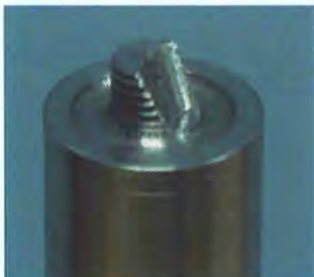
Figure 3.7: Flute tool geometry used to make the FSW.
