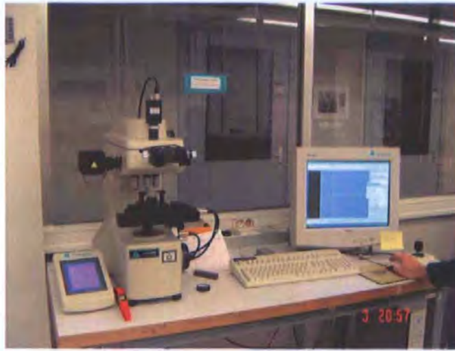
Figure 4.16: Buehler Micromet 5103 micro hardness tester at FAME38 in Grenoble, France.
