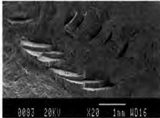
Figure 2.46: Planar facets observed on a bend fatigue specimen 1 .
