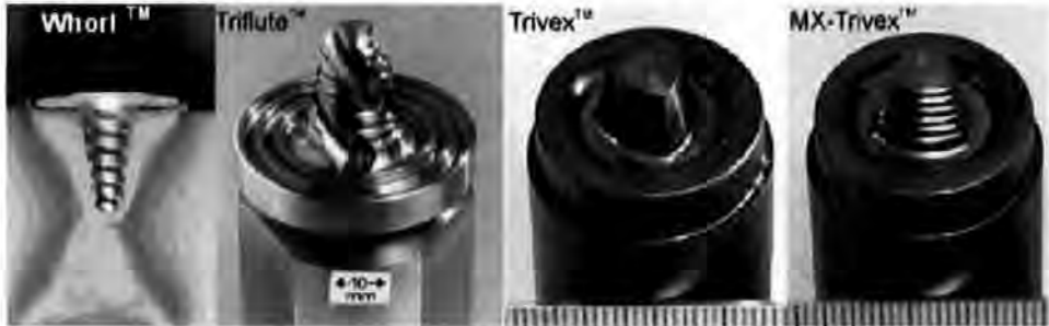
Figure 2.9: Whorl TM , Triflute TM , Trivex TM and MX Trivex TM tool designs.
