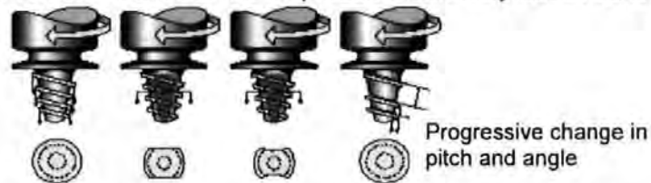
(a) Oval shape (b) paddle shape (c) Re-entrant (d) Changing spiral form
