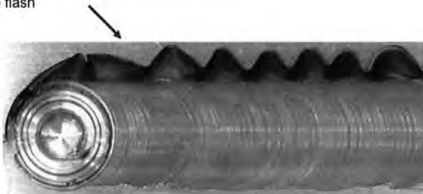
Figure 2.13: Side flash obtained during a trial weld at the Nelson Mandela Metropolitan University 1 .
