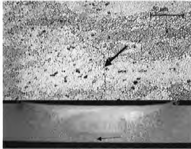
Figure 2.45: Root flaws indicated by the arrow 1 .
