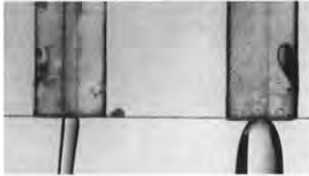
Figure 1.46 - Die swell effect. On flowing out of a capillary tube, a stream of viscoelastic liquid increases in diameter by 200 %, while a Newtonian liquid (on the left) shows a contraction of its diameter.
