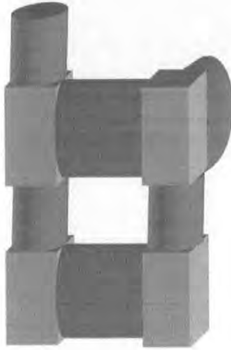
Figure 5.9 - Anisotropic structure showing throats with elliptical cross-section and rod-like pores with rectangular cross-section.
