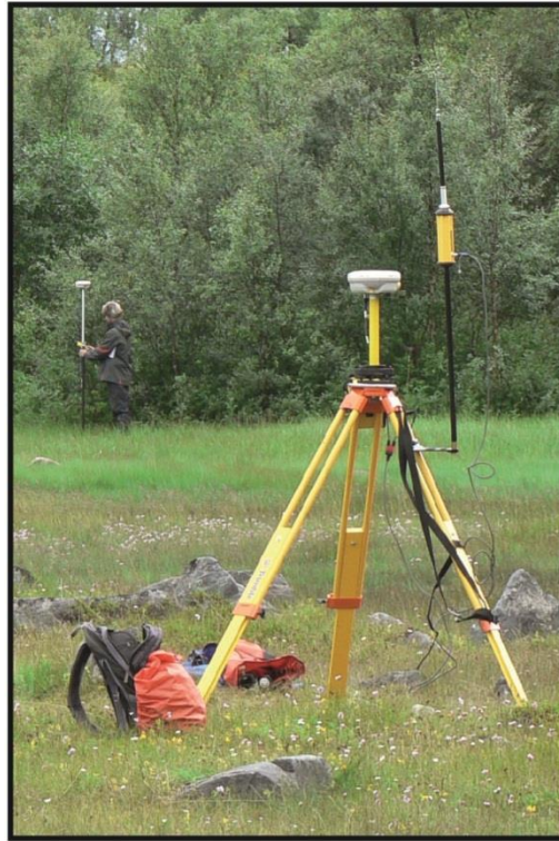
Figure 3.3 Foreground: Trimble DGPS RTK base station and antenna; background: Trimble Rover GPS
