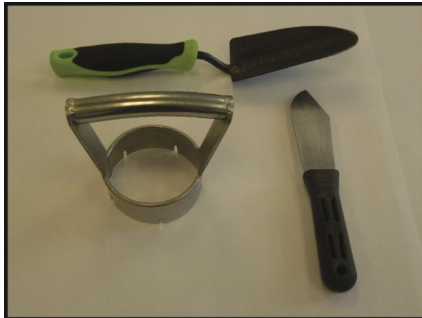
Figure 3.6 Turf cutter and surface sampling tools
