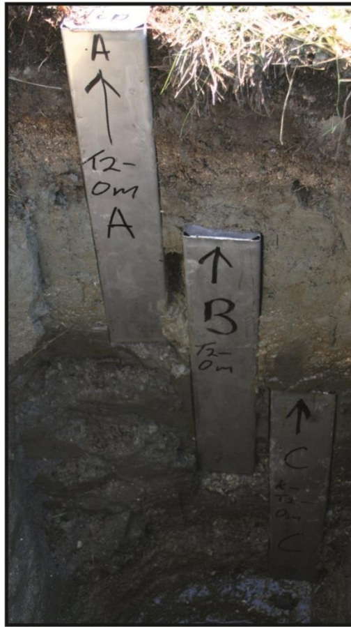
Figure 3.8 Example of monolith tins being used to collect fossil sediments from a dug pit
