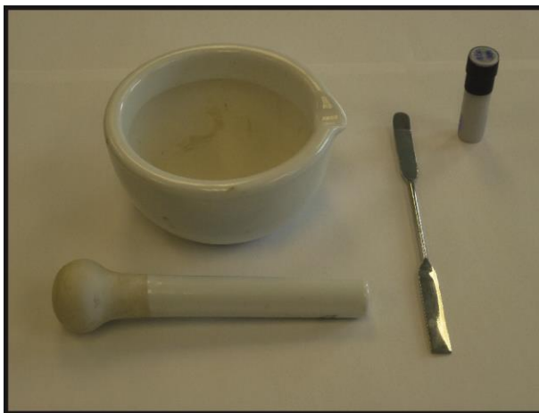
Figure 3.9 Tools used to prepare samples for radionuclide dating and a packed vial
