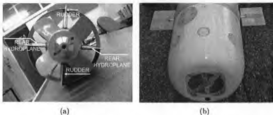
Figure 3.2: (a) Rudder and rear hydroplanes, (b) front hydroplanes
