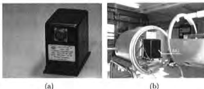
Figure 3.11: (a) Watson Industries Ltd. inertial measurement unit, (b) mounted inertial measurement unit
