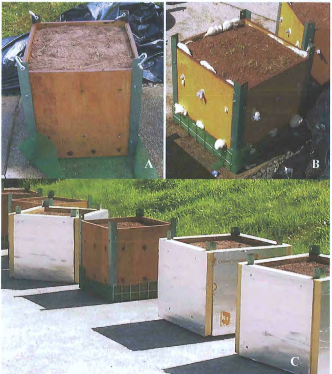
Figure 2.11. Lysimeter preparation: (A) six holes drilled into each side of lysimeter casing; (B) expanding foam injected into holes to prevent water flow between soil monolith and casing; (C) insulation attached to outside of the casing.
