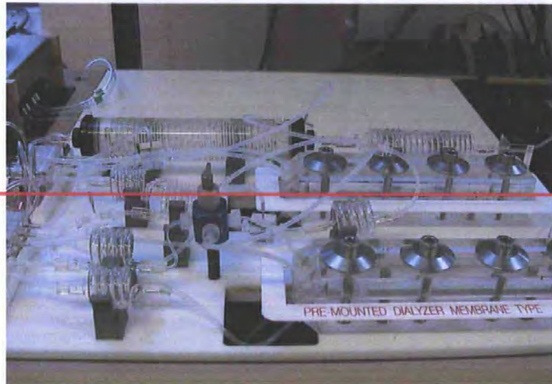
Figure 5.12. Skalar SANS PLUS chemistry unit. The manifold used for nitrate segmented flow analysis at IGER is below the red line.
