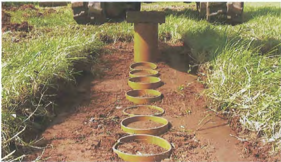
Figure 2.6. Extraction of intact cores of topsoil from the Crediton series.
