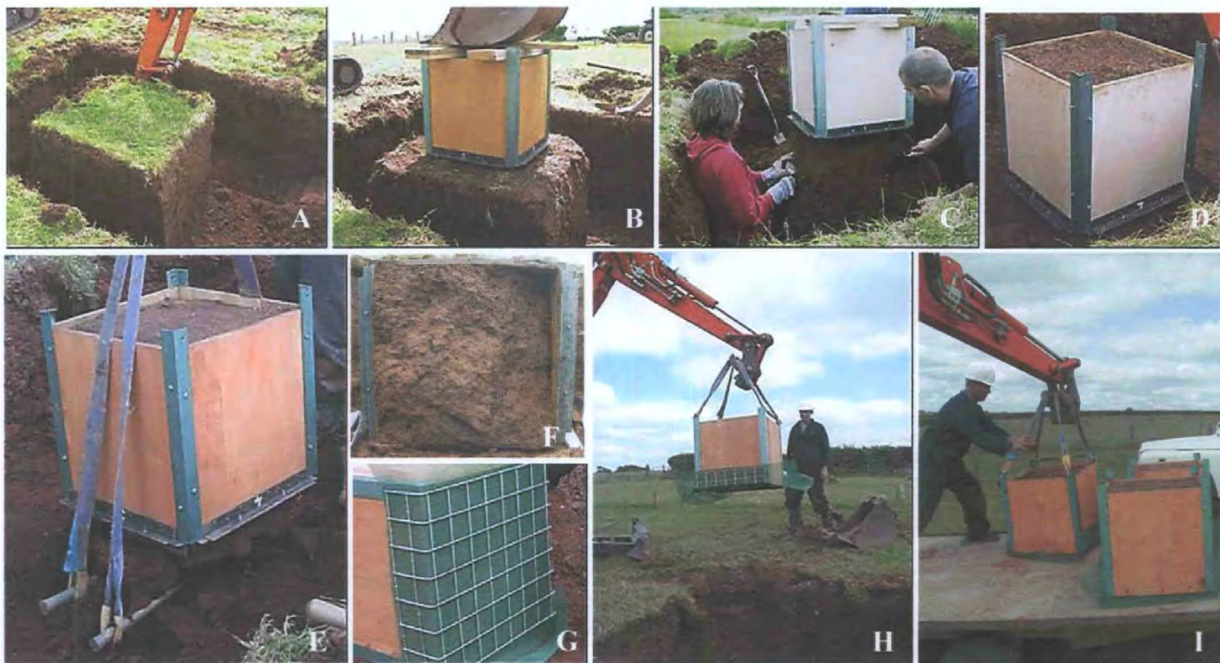
Figure 2.10. Lysimeter extraction: (A) trench dug around monolith; (B) lysimeter casing placed on monolith and gently pushed with bucket of digger; (C) soil and large stones removed from around cutting plate; (D) lysimeter casing filled; (E) lysimeter detached from bulk soil; (F) base of monolith trimmed; (G) nylon mesh and metal grid attached to base of casing; (H) intact lysimeter extracted with digger; (I) lysimeters placed on trailer for transportation.
