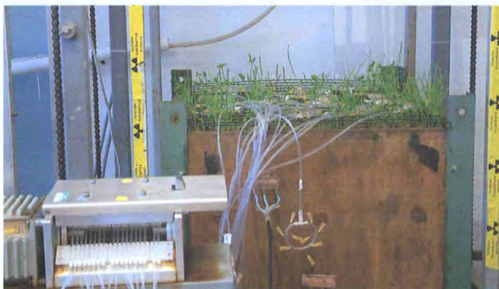
Figure 5.4. Simulation of rainfall and application of tracer solution to the surface of the soil block using a peristaltic pump attached to tubing and an array of 10 needles for fine delivery.
