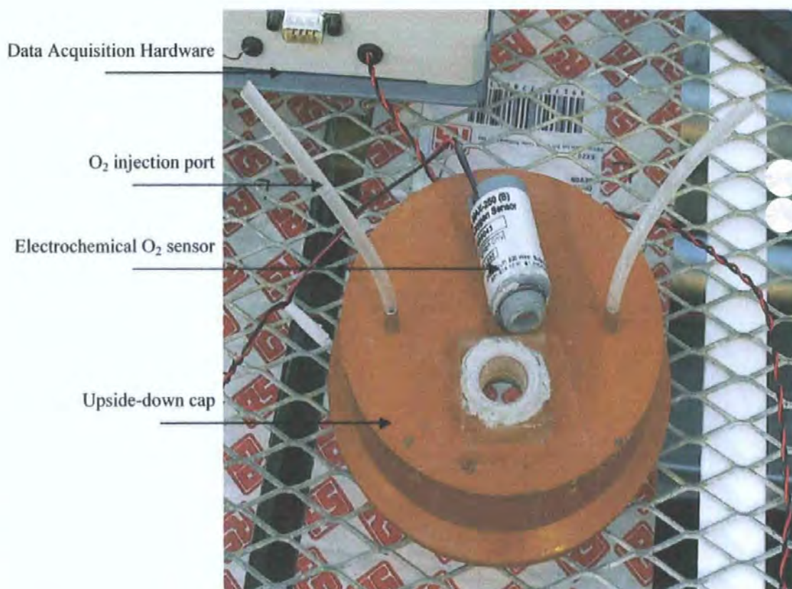
Figure 3.23. The equipment turned upside-down: machined plastic cap, with oxygen sensor (shown unscrewed from the plastic cap) and oxygen injection ports.
