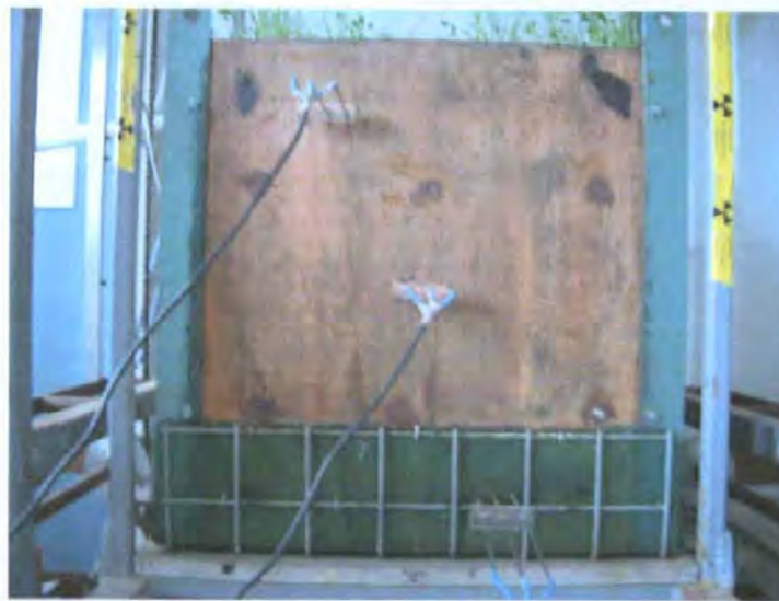
Figure 5.9. A mounted sample with three-inserted TDR trident probes as shown schematically in Figure 5.8.
