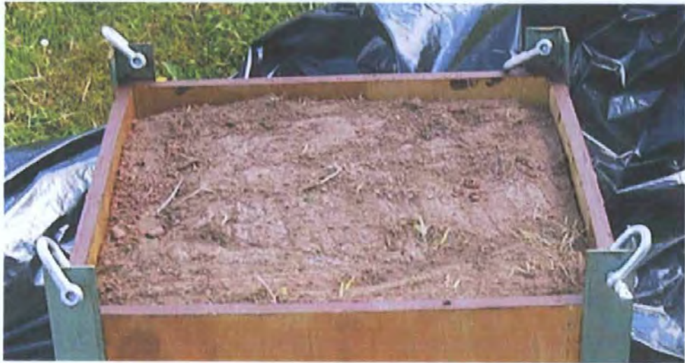
Figure 2.7. Assembly for lifting the lysimeter casing.
