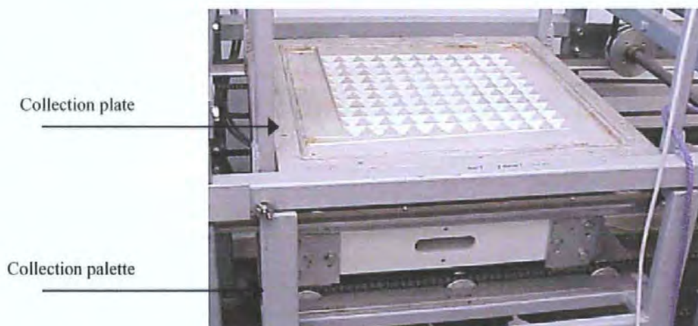
Figure 5.6. Precision-machined collection palette aligned with the sample collection plate.
