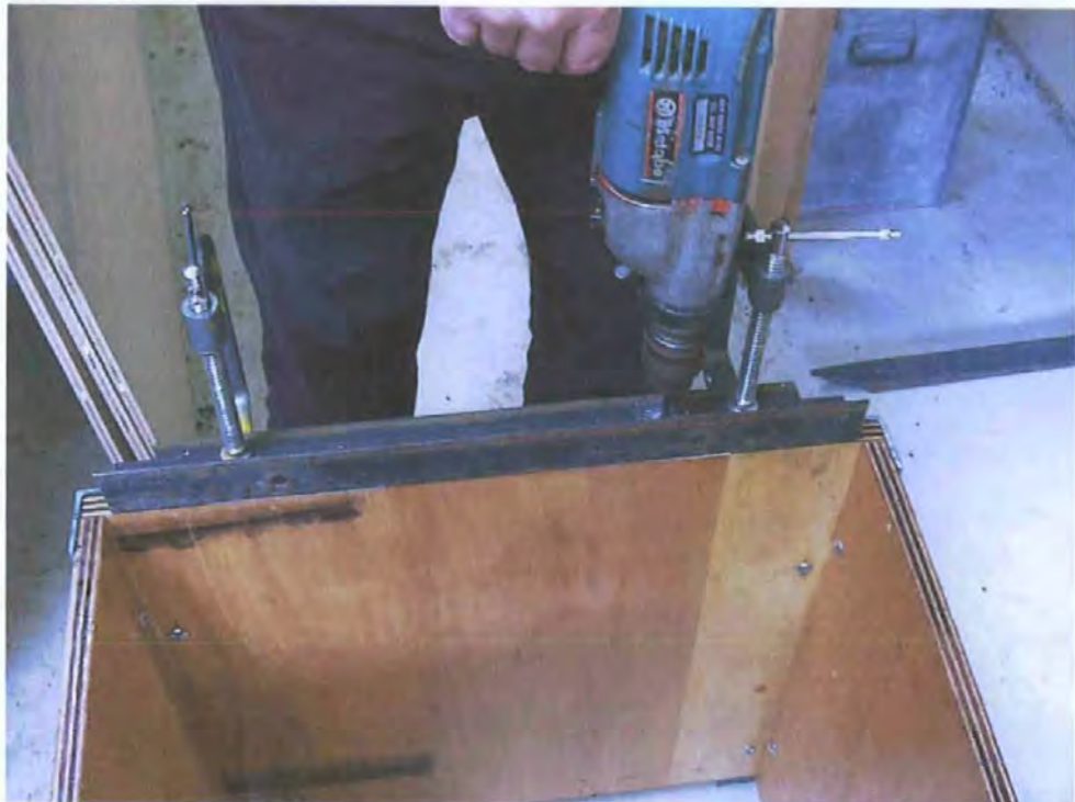
Figure 2.8. Metal cutting plate attached to the base of the lysimeter casing.
