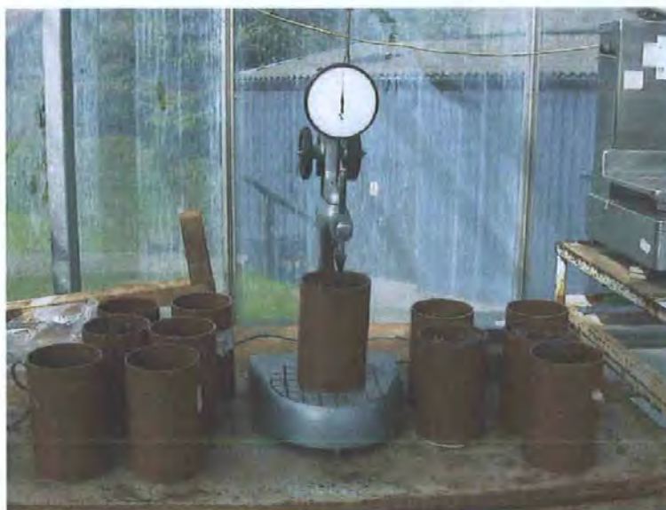
Figure 3.9. Drop-cone penetrometer to determine the stability of aggregates when exposed to external mechanical stresses, and resistance to forces that cause compaction.
