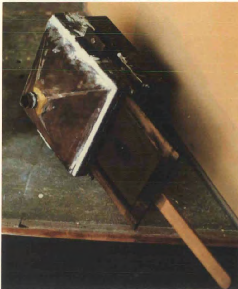
Fig. 2.15 The Box Cassette Filter (BCF) with Sliding Filter Holder
