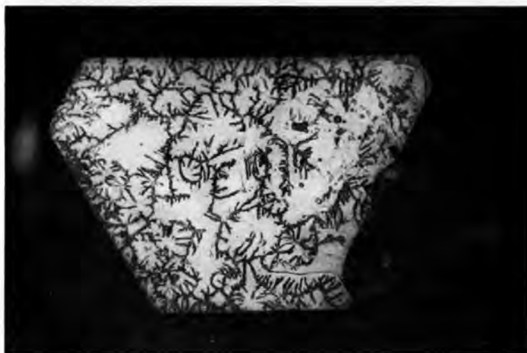
Reflection optical micrograph of a (111) face of a typical MBS 35/40 diamond as supplied.
