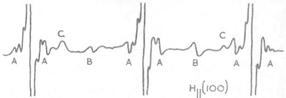
E.S.R. SPECTRUM OF NITROGEN DONORS IN DIAMOND, GROUP A LINES DUE TO ^{13}\text{C} (CENTRES II, III, AND IV,); GROUP B LINES DUE TO NITROGEN QUADRAPOLE MOMENT; GROUP C LINES DUE TO ^{15}\text{N} .
