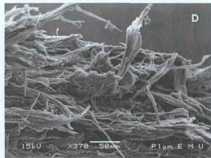
Figure 5.10 SEM image of fracture surface of tension tests of hoof horn of the sole area perpendicular to the direction of the tubules, horn with great elasticity showing fibre pullout of intertubular horn (Picture A x 750, scale line = 20µm; picture B and C x 650, scale line = 20µm and picture D x 370, scale line = 50µm).
