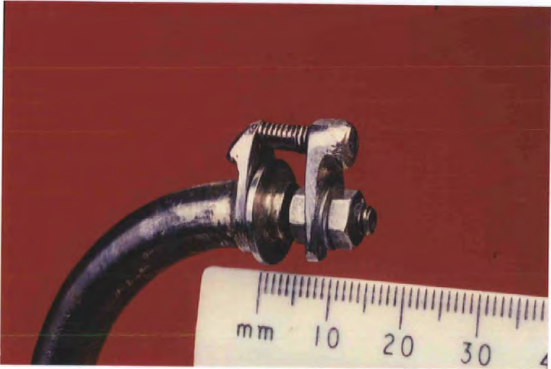
Plate 1 The spray head attachment used to evenly disperse the solvents with the oncoming exhaust.
