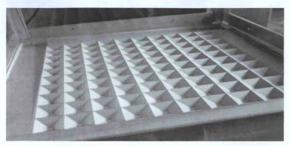
Figure 4.2 Sample Collection plate top view.
