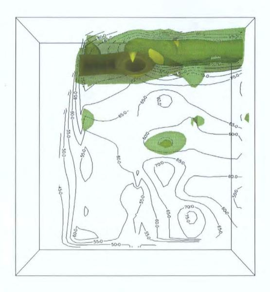
Figure II.6 Sollom Oil Distribution Profile View.
