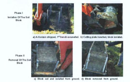
Figure 2.13 a, b, c, & d. Stages of soil block extraction.
