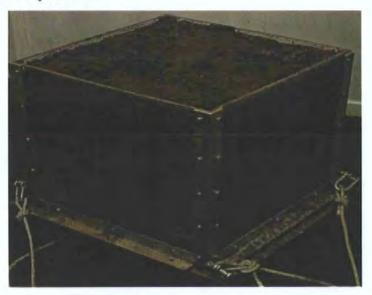
Figure 2.14 The extracted soil block awaiting mounting onto the lysimeter.
