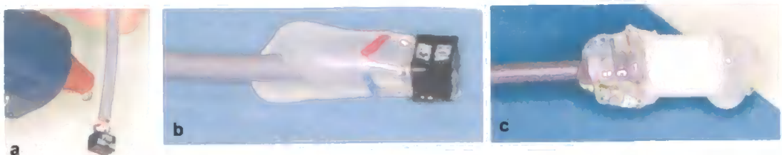
Figure A6: Waterproofing of the CAPMON sensor
