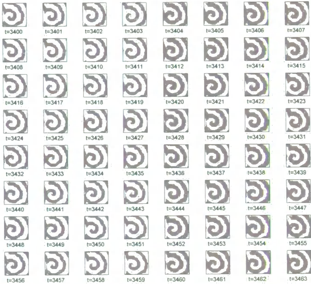
Figure 2.14: Spiral wave produced with a = 3 , initialized with p = 0.5 and initial thresholds \{4,5,6\} . The period of this spiral wave is 64.
