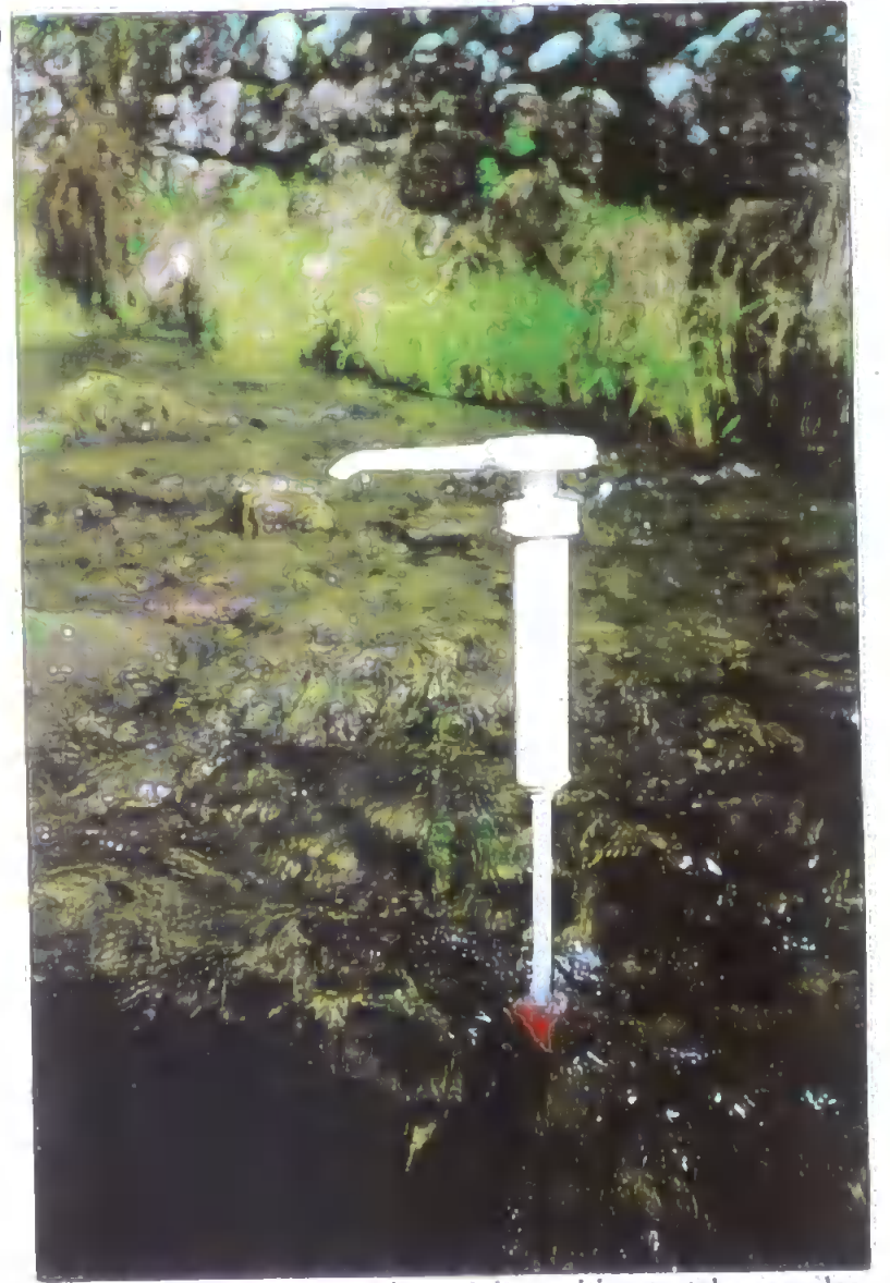
Plate 2.1. A) Hand pump and tube used to obtain interstitial water samples (Arrow points to a hole in the tube) B) Hand pump in position to take samples.
