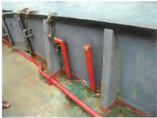
Fig. 5.10 Improper securing of a boarding ladder
