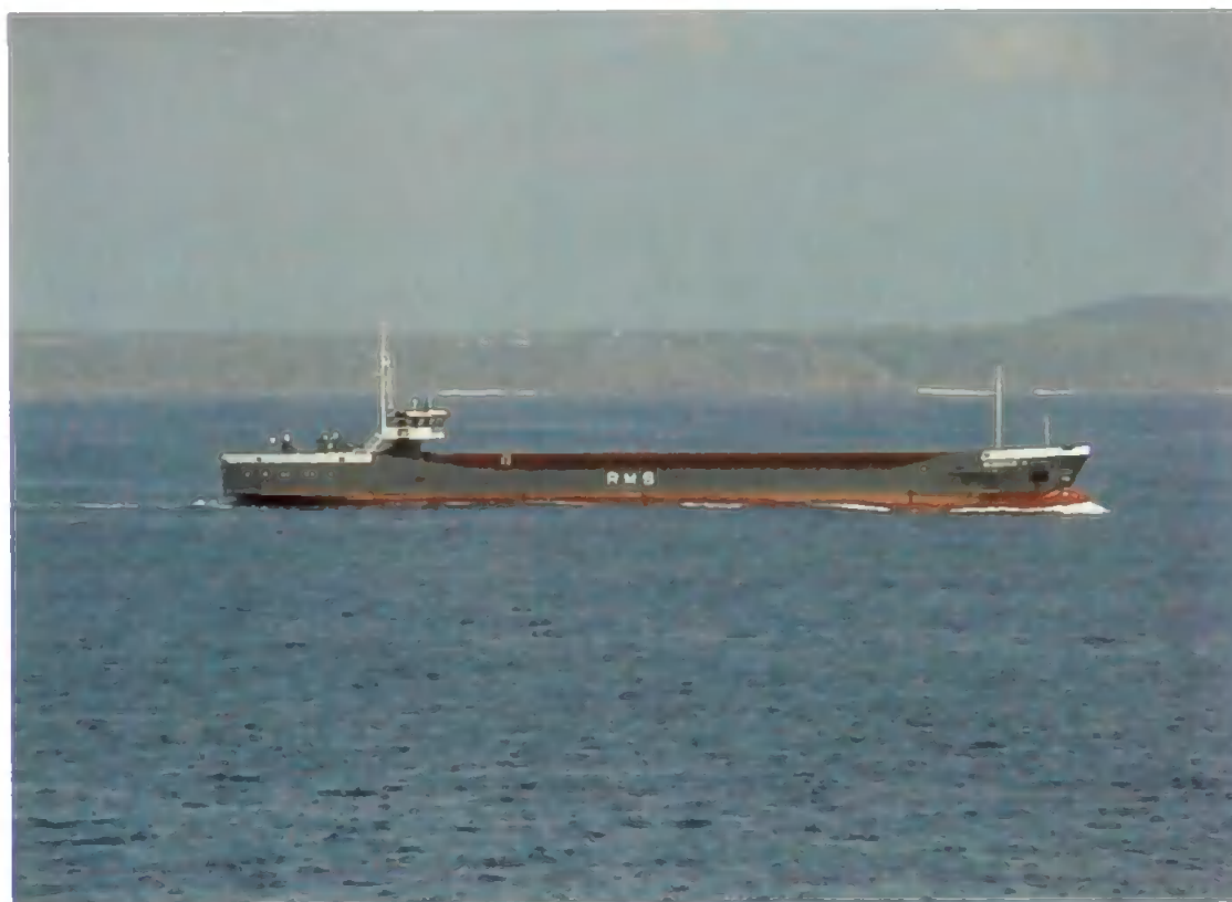
Figure 6-13 River-sea ship with hydraulic wheelhouse
