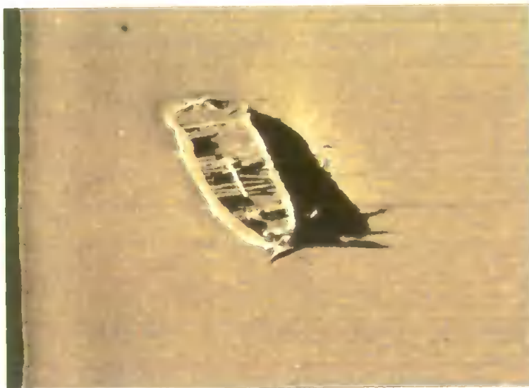
Figure 5.8: Typical SSS image (500 kHz) of a shipwreck on a 75-metre range collected with a Klein Side Scan Sonar System 3000. (Source: Klein Associates Inc.)
