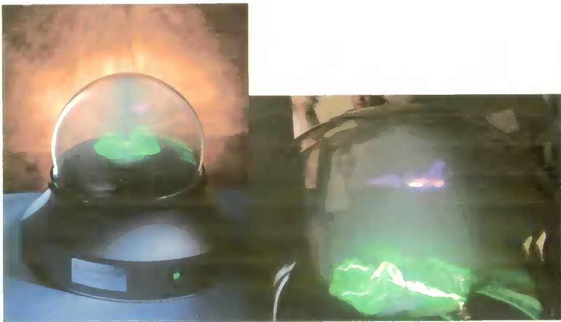
Figure 4.14: An example of a volumetric spherical display. A pink fighter airplane is visualised above the green terrain. In the right picture the fighter plane is visualised in side view. (Source: Actuality Systems Inc.)
