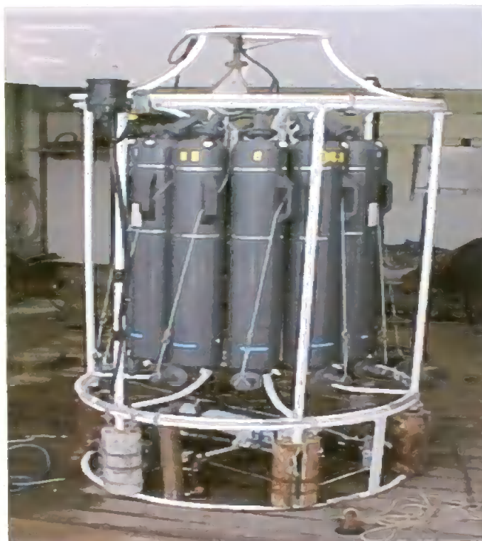
Figure 5.5 Sea Bird SBE 32 Carousel Water Sampler on the deck of the JCR with conductivity-temperature-depth (CTD) instrumentation fitted.
