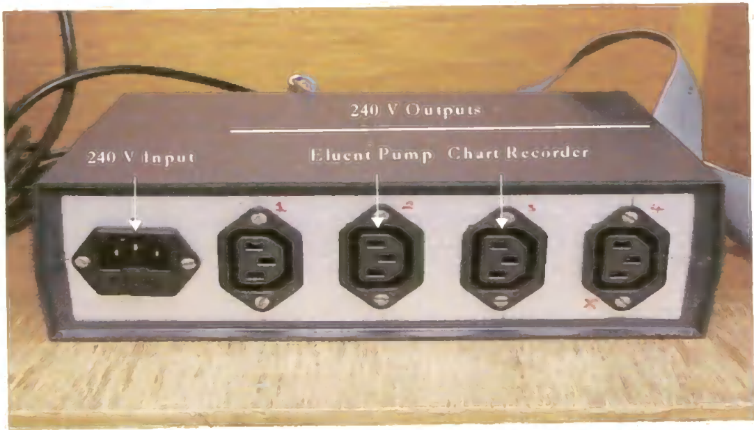
Figure 4.4 Rear Panel of Relay Box - Input and Output Connections
