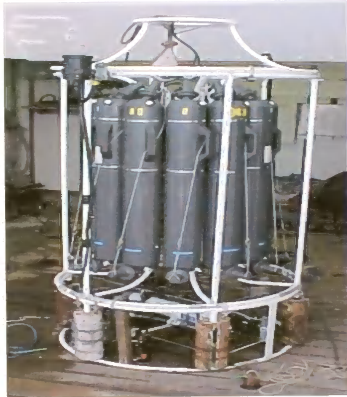
Figure 1.5 Sea Bird SBE 32 Carousel Water Sampler with a high quality, epoxy coated stainless steel carousel frame, fitted with 12 grey poly(vinyl chloride (PVC), Teflon® lined, free flushing water sampler bottles (Ocean Test Equipment Inc., model 110, 12 L capacity) fitted with latex tubing spring closures, with silicone 'O' rings and seals and HDPE plastic drain valves to minimise metal contamination.
