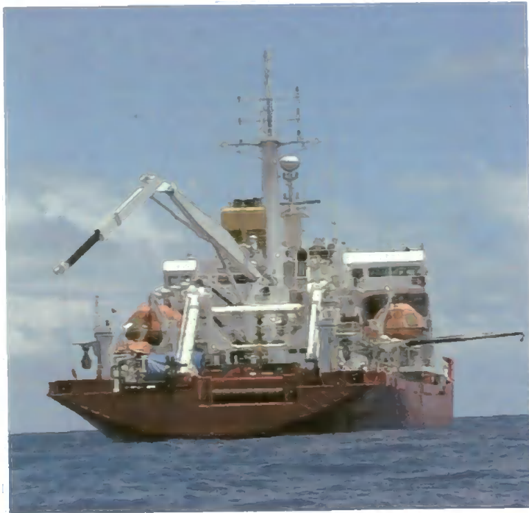
Figure 5.2 RRS James Clark Ross on Station. The CTD was deployed from the remotely operated arm seen on the port side of the vessel.
