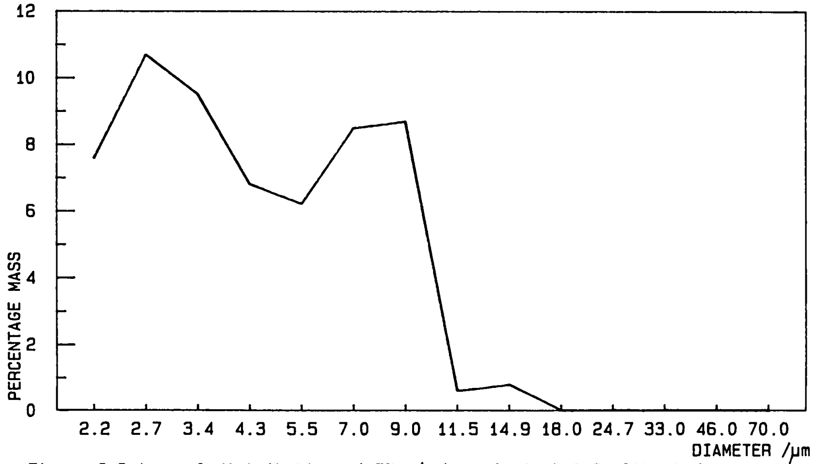
Figure 2.9 Aerosol distribution of 5% m/v benzyl alcohol Zeolite A slurry
