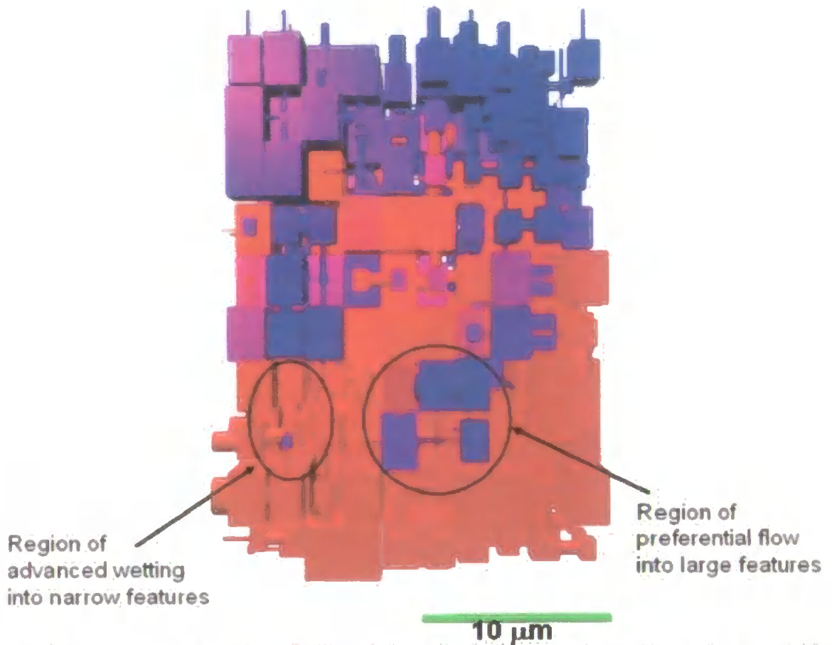
Fig. 8. 25. Simulated absorption of oil into OpacarbA40-CL using the estimated aspect factor ( \alpha=1.5 ) at 0.1 seconds, but ignoring inertial effects (Lucas-Washburn equation).
