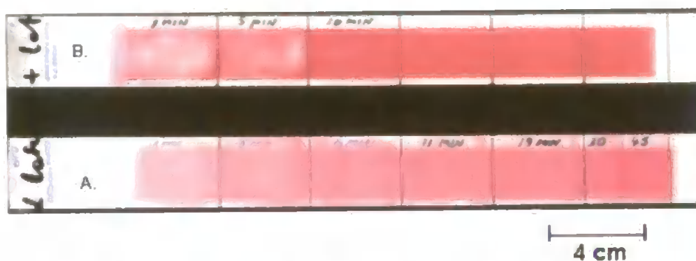
Fig. 3. 7. Example of the ink stain obtained from the Speswhite (A) and Amazon (B) coating strips at various elapsed times (shown in minutes).
