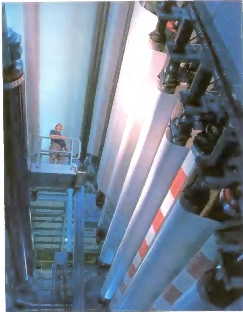
Fig. 1. 13. Example of a Supercalender machine ( www.repap.com ).
