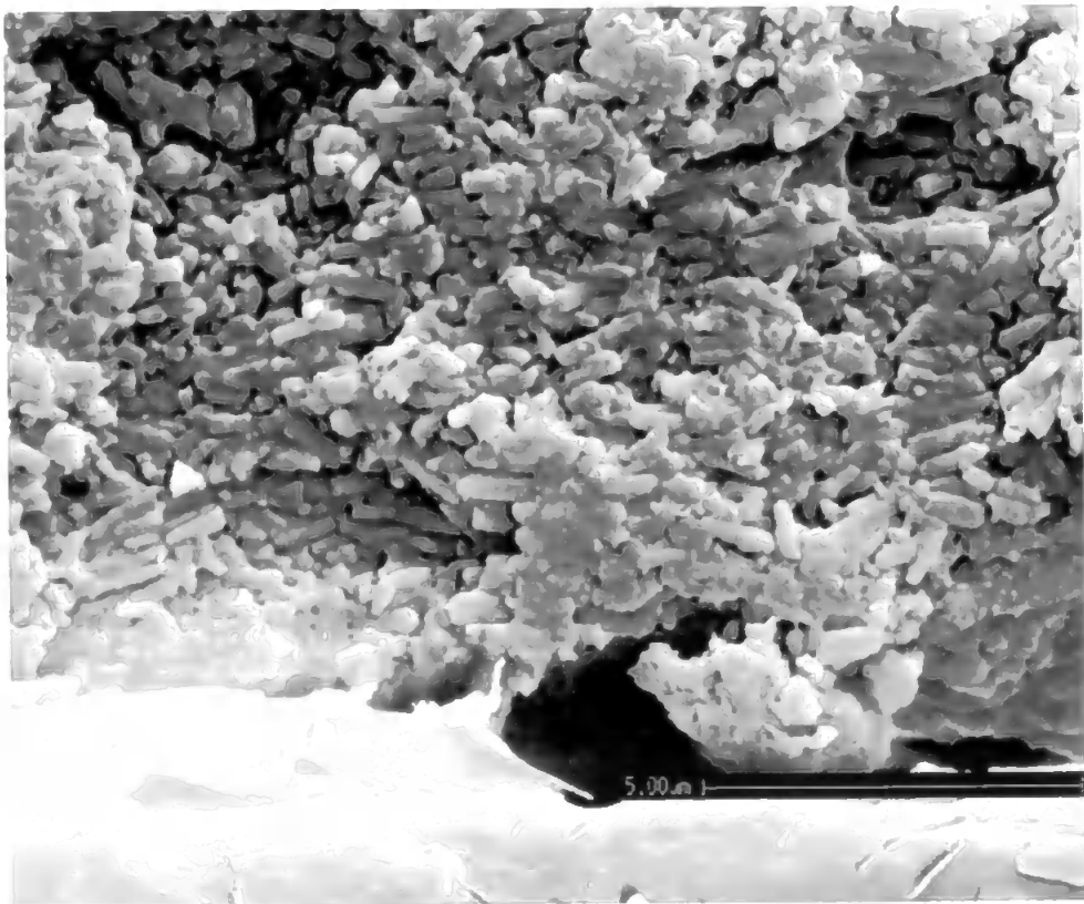
Fig. 5. 11. OpacarbA40-CL: scanning electron micrographs of resin-embedded cross-sectional scan. Scale bar: 5 \mu m.
