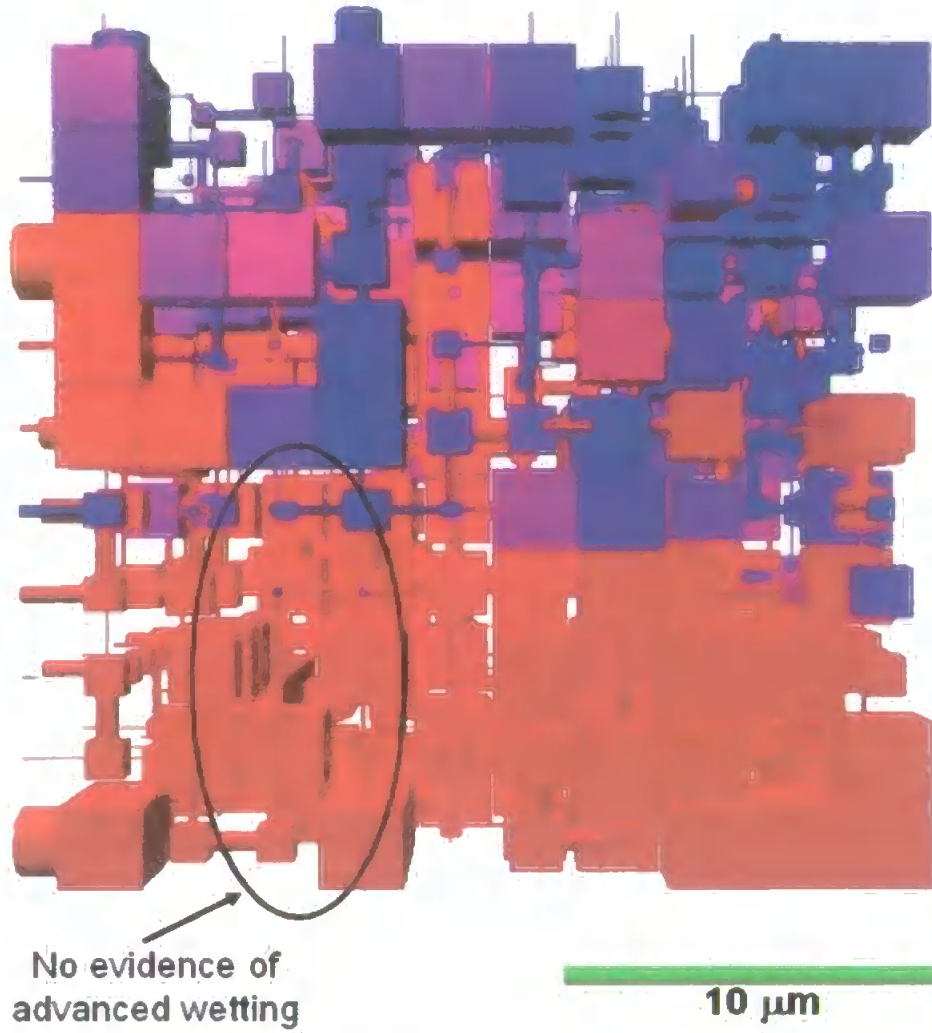
Fig. 8. 15. Simulated absorption of oil into Speswhite-CL control ( \alpha=1 ) at 0.1 seconds, including inertial effects (Bosanquet equation).
