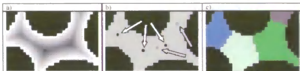
Fig. 2. 11. Erosion of void space – each successive erosion shown darker. b) Identification of pore centres as maxima of erosion contours (false maxima shown grey). c) Partitioned pore space (Toivakka et al. , 2000).
