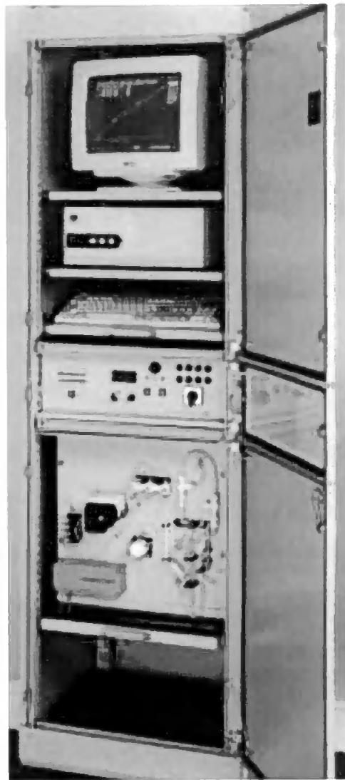
Figure 2.18. On-line mercury monitoring system
