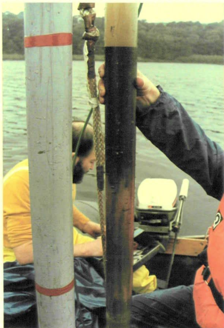
Plate 4.1: A 1m core taken using a Mackereth mini-corer. The marked difference in colour between the dark brown of Zone A and the red clays at the top of Zone B can clearly be seen. This type of corer causes considerable disturbance of the sediment structure.
