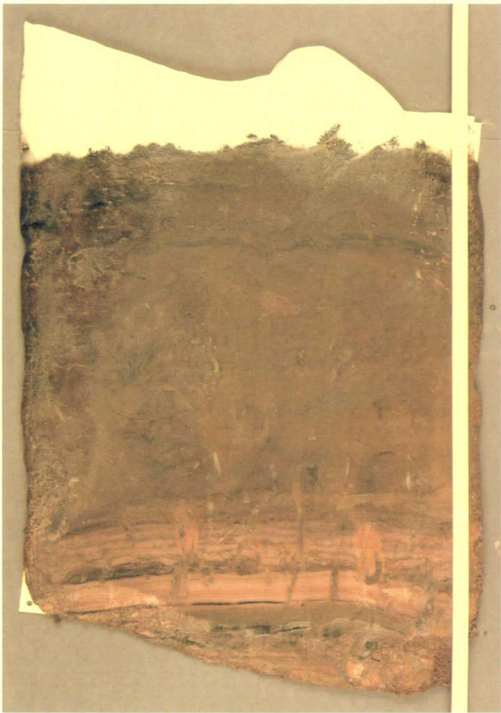
Plate 5.5: Core FBS12. The sample measures 31cm in width and approximately 37cm from the sediment-water interface to the base. The majority of Zone A has been considerably bioturbed, but some structure is still visible towards the sediment surface. The burrows of benthic fauna can be seen penetrating into the red clays which mark the top of Zone B.
