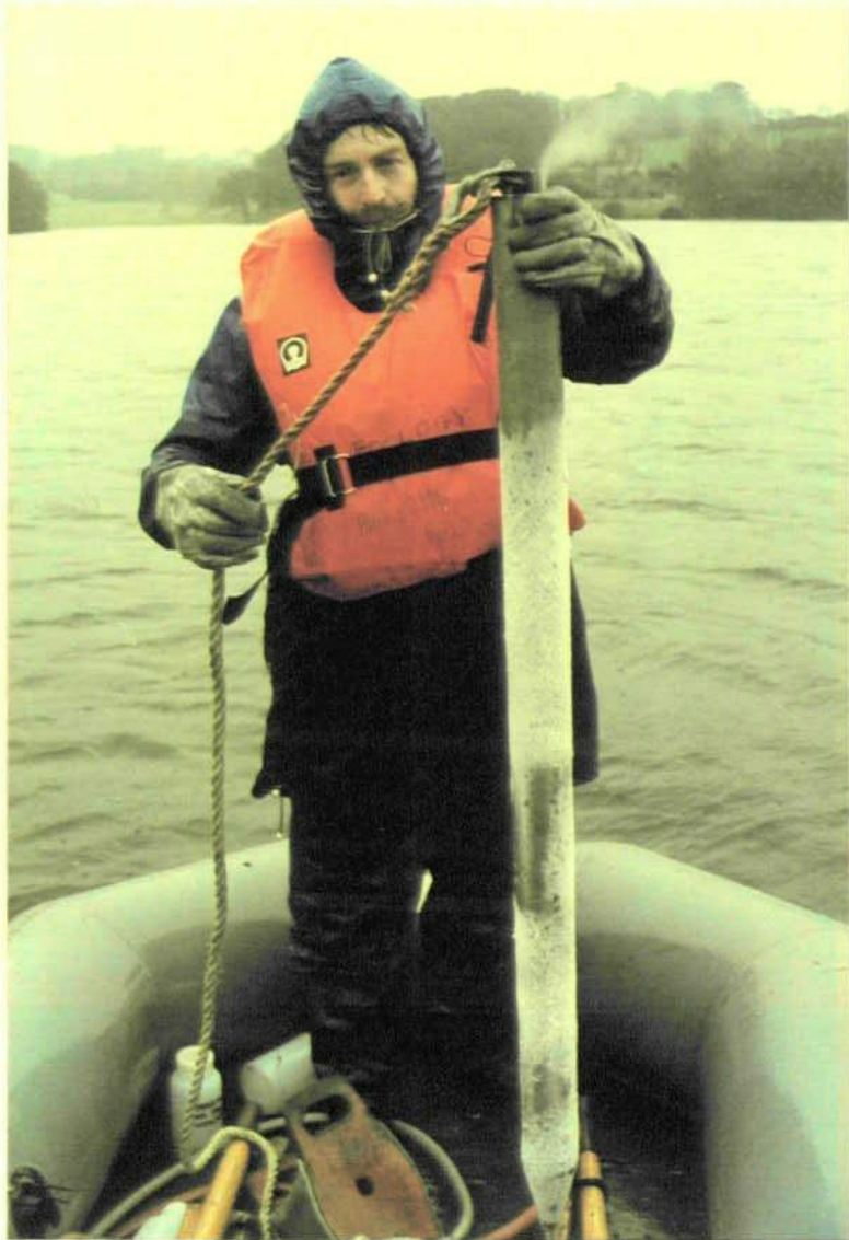
Plate 4.3: An 'Icy-Finger' sampler, packed with solid carbon dioxide and acetone, prior to sediment sampling.
