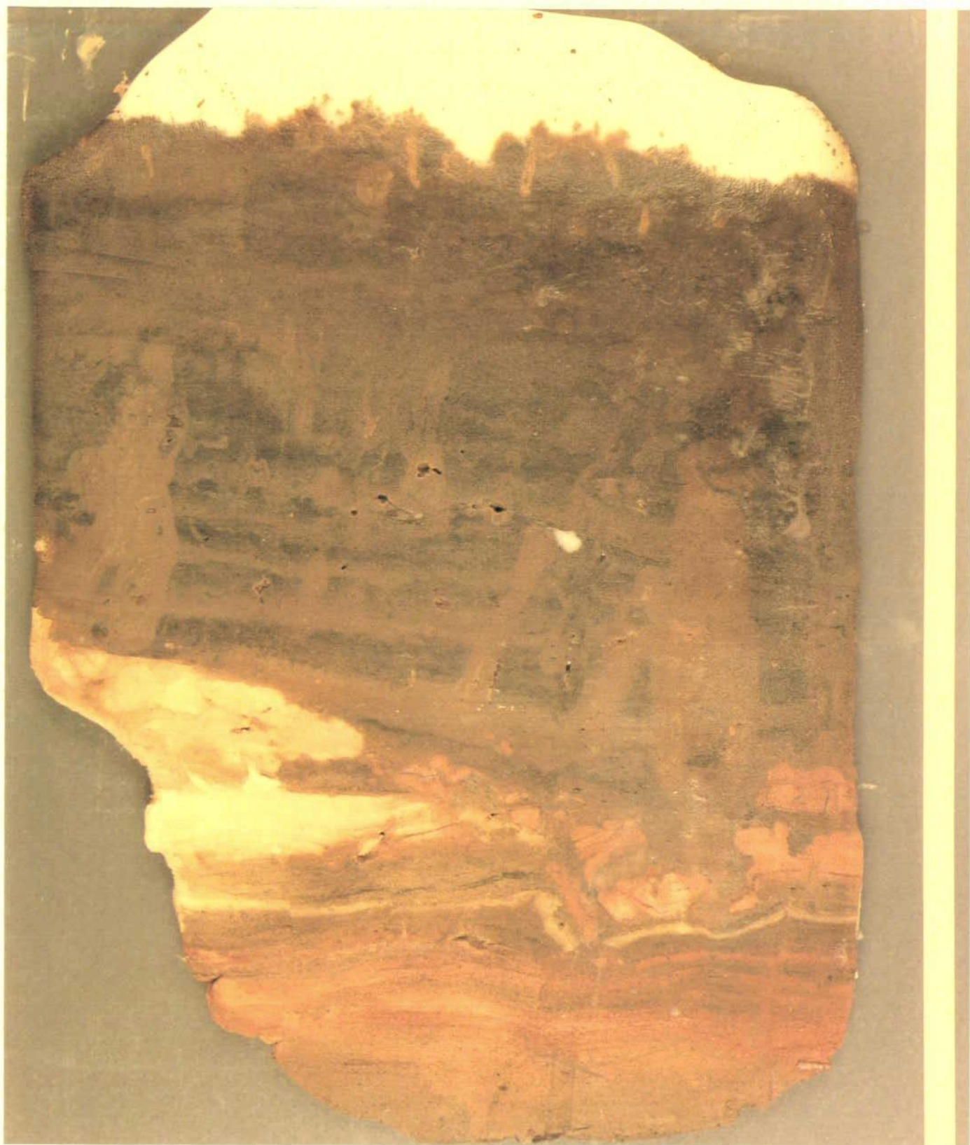
Plate 5.4: Core FBS3. The sample is 30cm wide and approximately 38.5cm from the sediment-water interface to the base. Zone A, above the red clay, shows considerable structure. However, the alternate brown and black layers are not annual in nature. Bioturbation can clearly be seen, with evidence of recent zoobenthic activity close to the surface.
