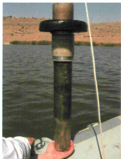
Plate 3.8 Messenger-operated gravity corer (Glew et al. , 2001) containing the NAR06 core section (summer, 2006).
