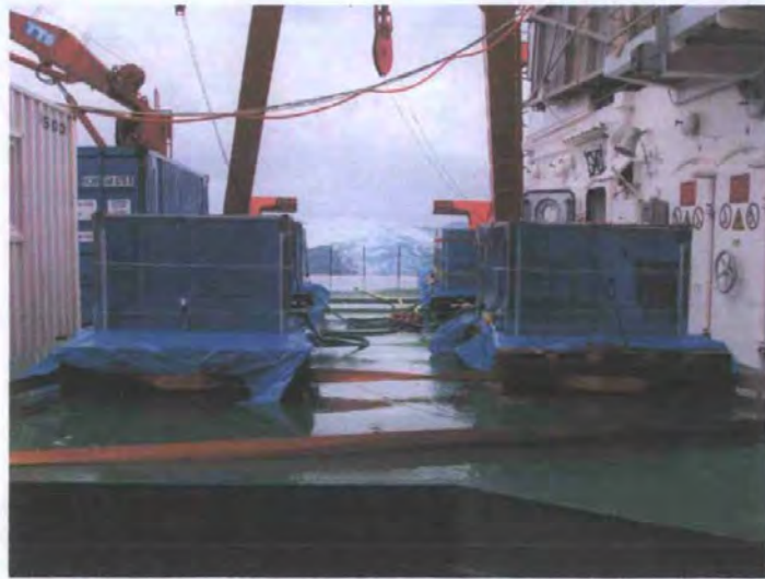
Figure 3.3 On deck incubator tanks used during dissolution studies. Light was attenuated to 20% of incident surface values using blue filters.
