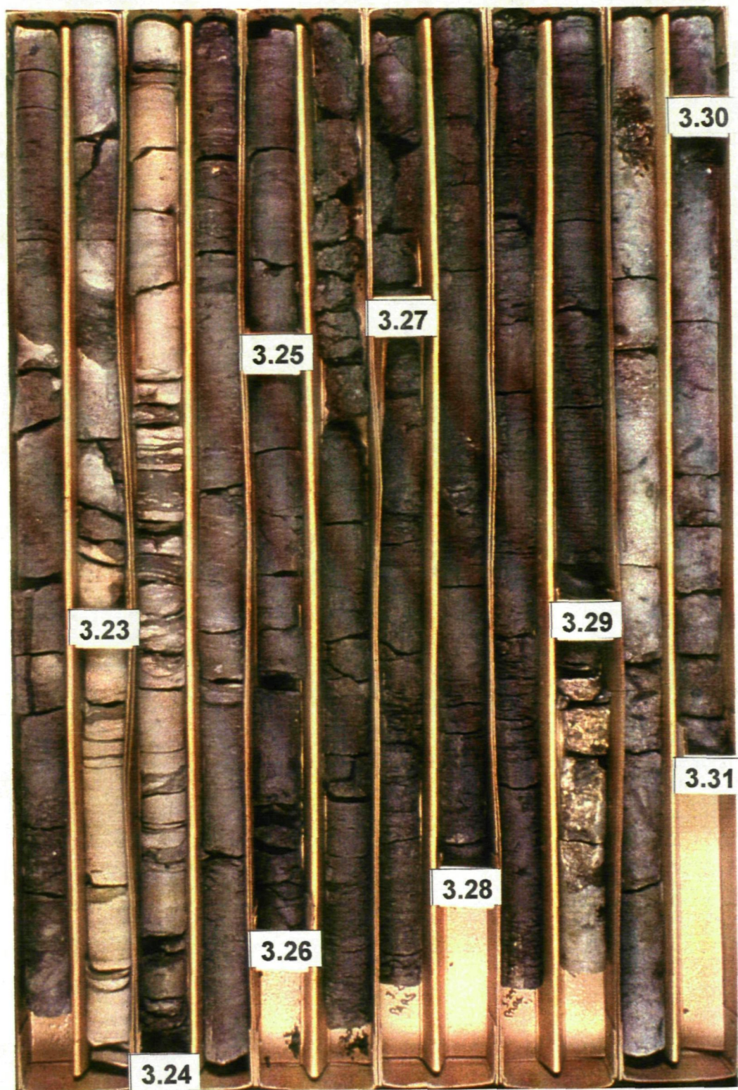
Figure 3.5. Hallett's Farm Borehole core photographs. Cores 3.23 to 3.31. The core numbers are situated at the base of each core and represent the following depths. Core 3.23 – 33.62m, 3.24 – 35.16m, 3.25 – 36.68m, 3.26 – 37.23m, 3.27 – 38.53m, 3.28 – 40.07m, 3.29 – 41.59m, 3.30 – 43.11m, 3.31 – 44.65m.
