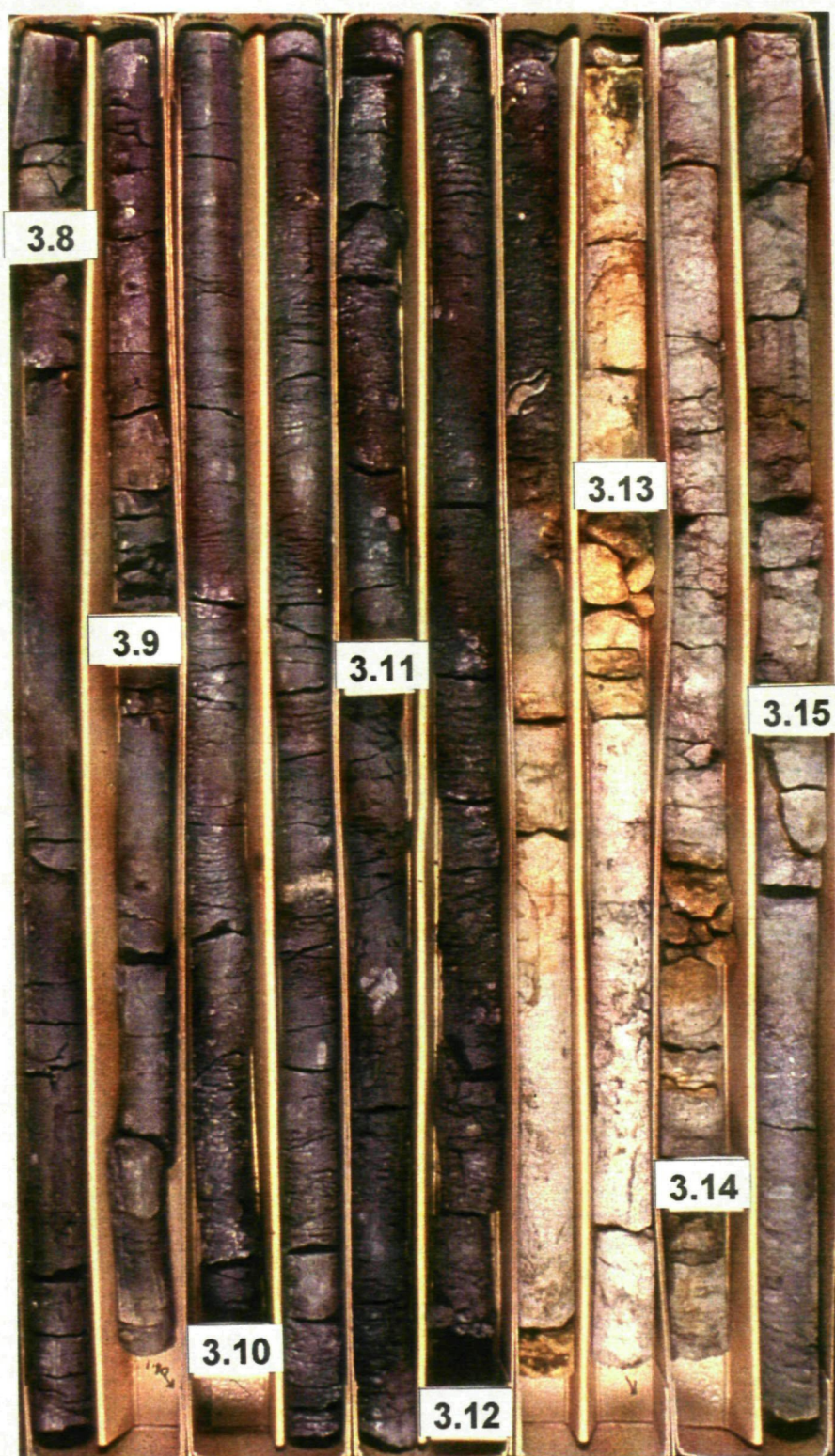
Figure 3.3. Hallett's Farm Borehole core photographs. Cores 3.8 ( pars ) to 3.16 ( pars ). The core numbers are situated at the base of each core and represent the following depths. Core 3.8 – 13.55m, 3.9 – 15.07m, 3.10 – 16.59m, 3.11 – 18.11m, 3.12 – 19.63m, 3.13 – 21.15m, 3.14 – 22.67m, 3.15 – 23.18m.
