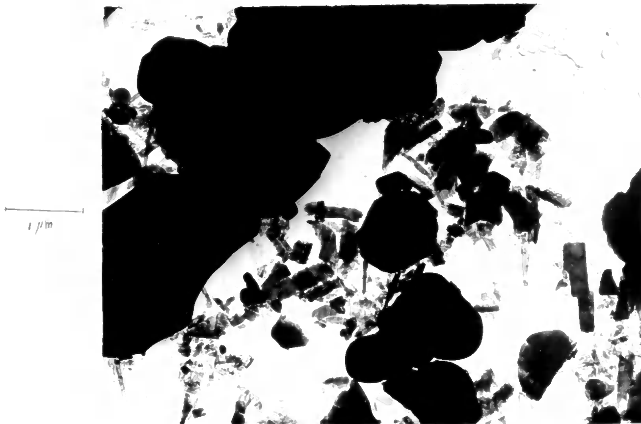
PLATE 4.3:1 Vanadium Nitride, Oxidised in Air at 500°C for 2 hours
