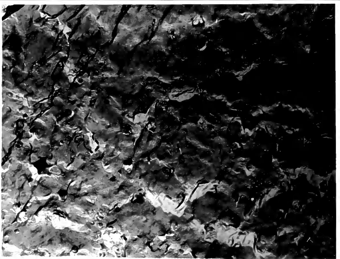
PLATE 3.1(a) I.M.I. 130 Nitride Coated for 8h at 1000°C.
