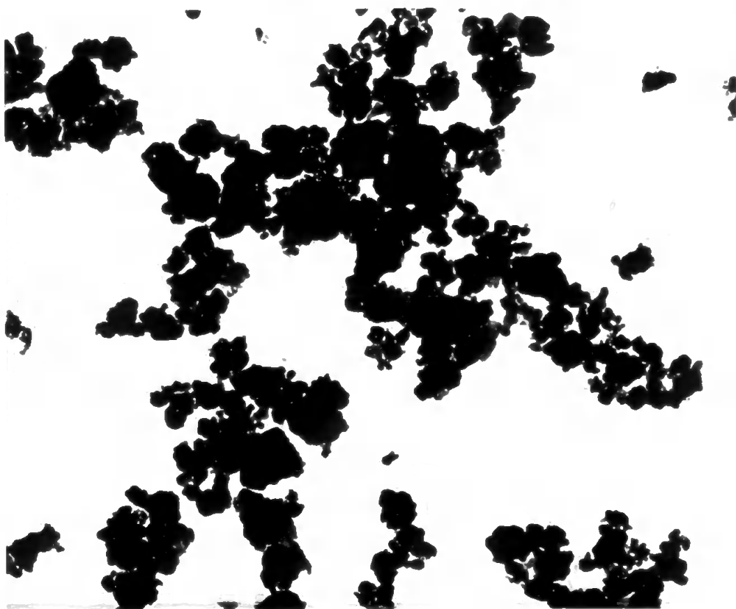
PLATE 5.2 Chromium Nitride, Oxidised in air at 1000°C for 5 hours
