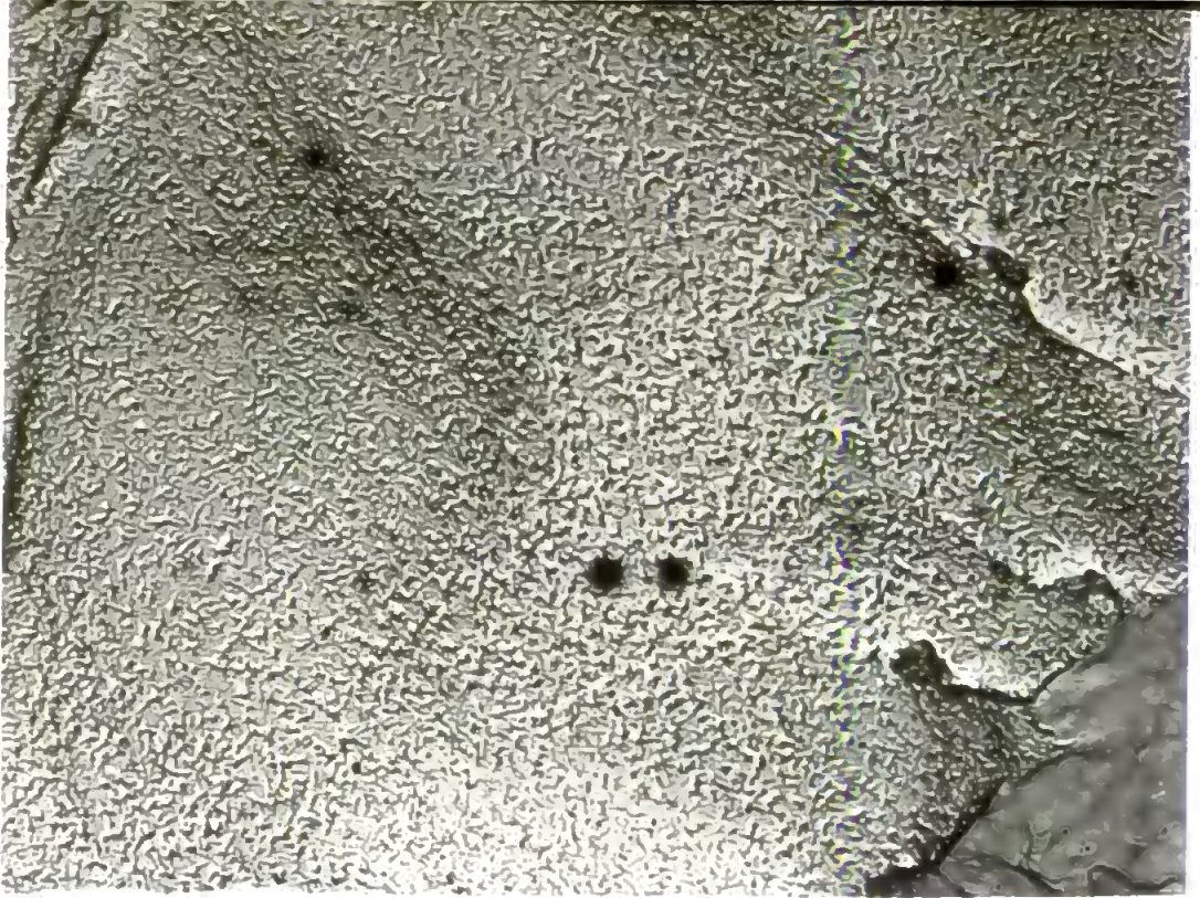
PLATE 3.2(a) I.M.I. 205 Nitride Coated for 8h at 1030°C.
