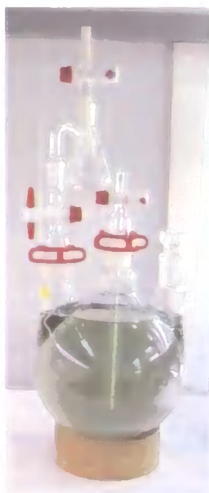
Figure 4.7: Purpose-built culturing flask used for ^{13}\text{CO}_2 incorporation experiments.
