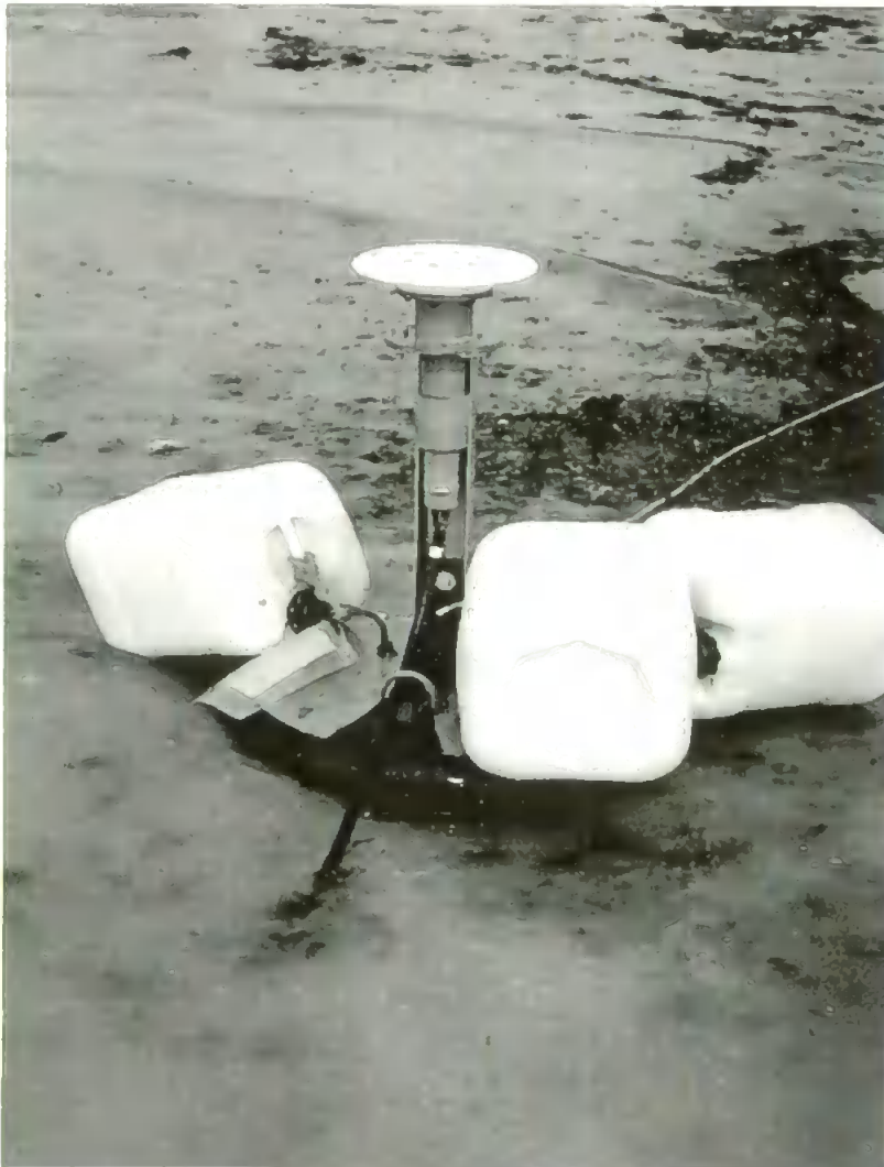
Plate 3.3 Pressure transducer and its housing prepared for the offshore deployment
