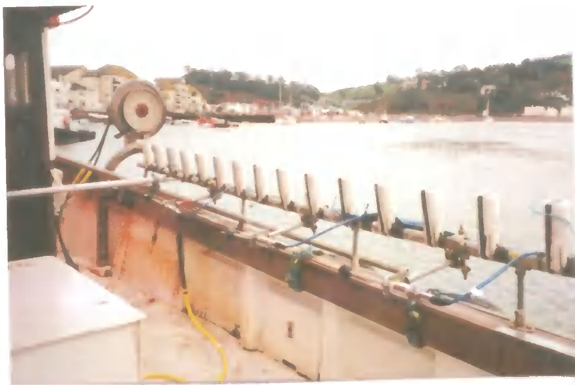
Plate 3.3: ETS with EMCM's attached before deployment in the field.
