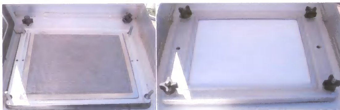
Figure 5.5. a) Anodised aluminium filter holder, b) Filter ready for sampling, secured by the frame.
