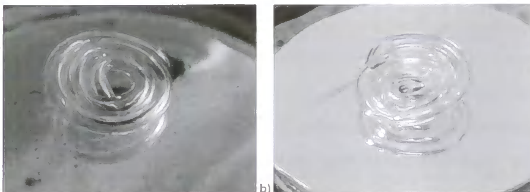
Figure 2.16. a) PMT opened with flow cell. b) detail of flow cell and mirror.
