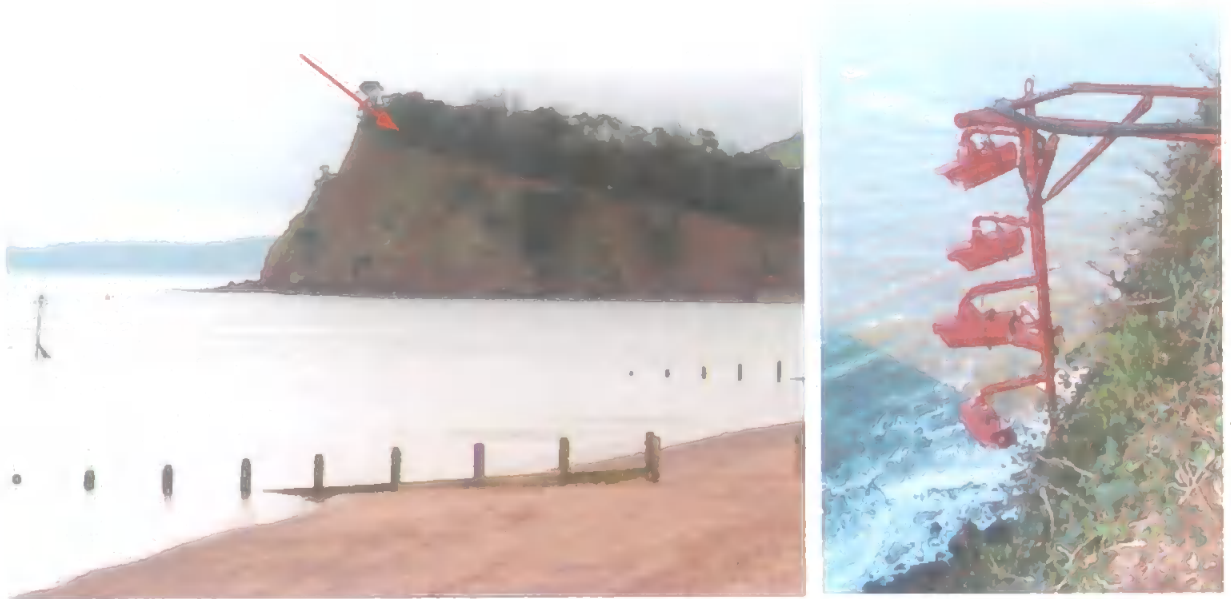
Figure 3.9. The Ness, with the arrow indicating the position of the Argus video cameras, detailed in the right hand side.
