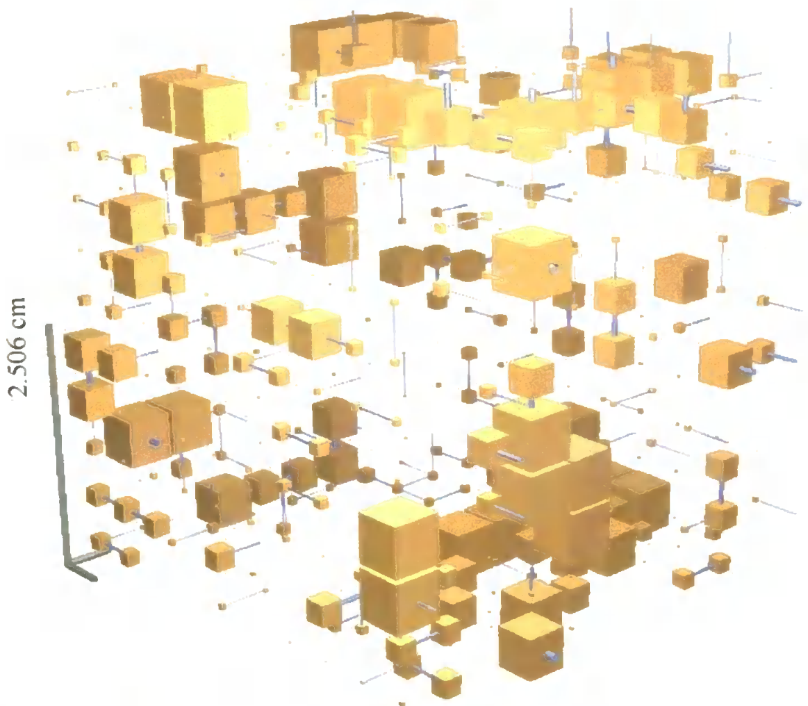
Figure 6.10: Compacted Sandy Clay Loam. Normalised porosity 7.74 %.
