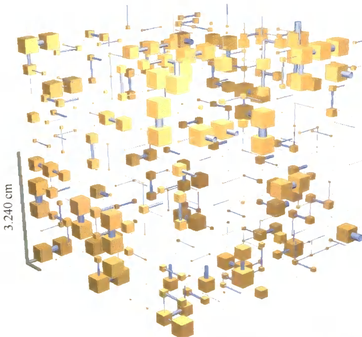
Figure 6.6: Simulated Clay Structure. Normalised porosity 4.03%. Unit cell length is 3.240 cm. Small scale bar is the pore row spacing of 3240 \mu\text{m} .
