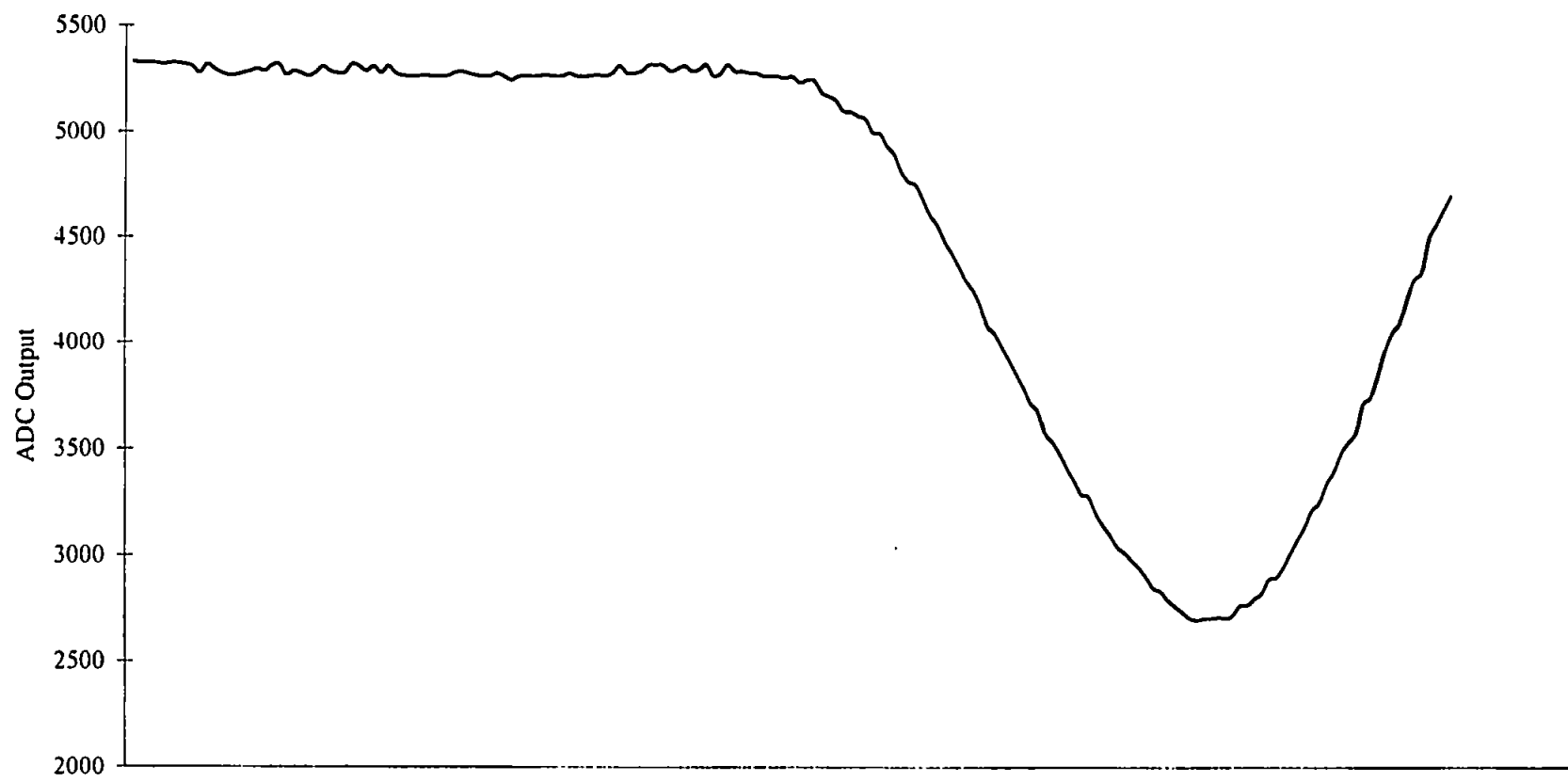
Figure 4.5. Typical peak from a 2.0 \mu\text{M} Nitrite-N standard injection (LED set at maximum power)
