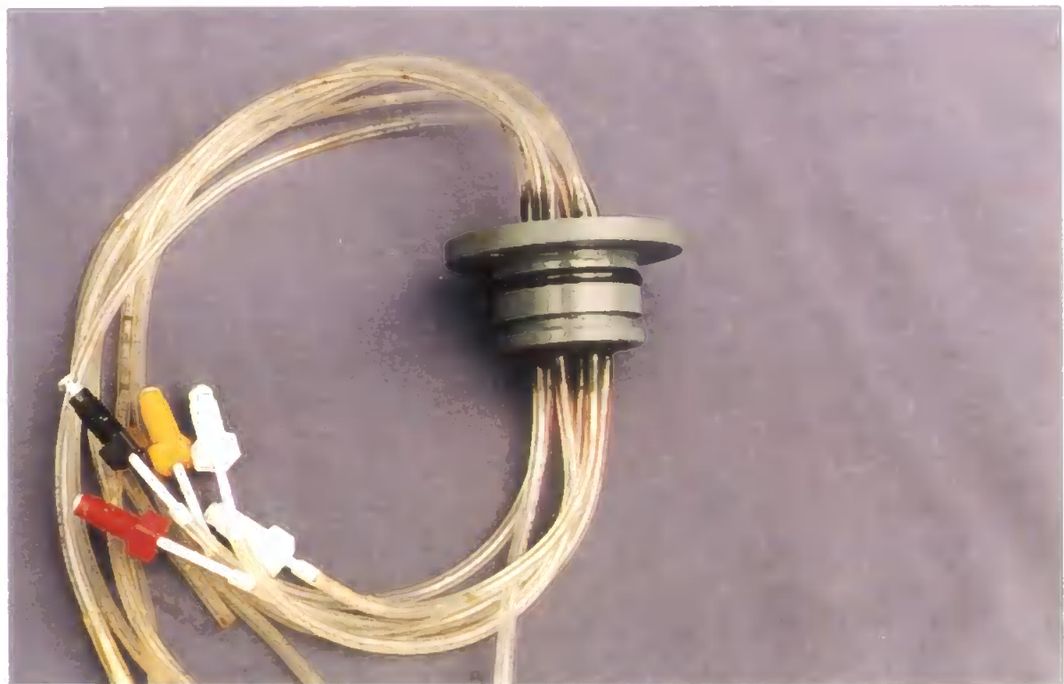
Figure 3.43. Detail of tube entry device showing 'O' seals
