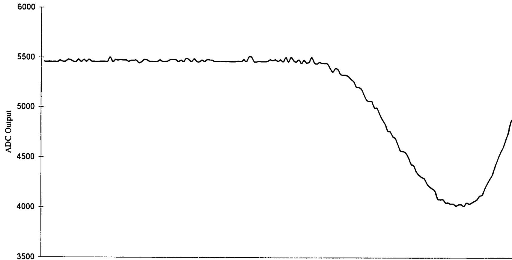
Figure 4.4. Typical peak from a 1.0 \mu M Nitrite-N standard injection (LED set at maximum power)
