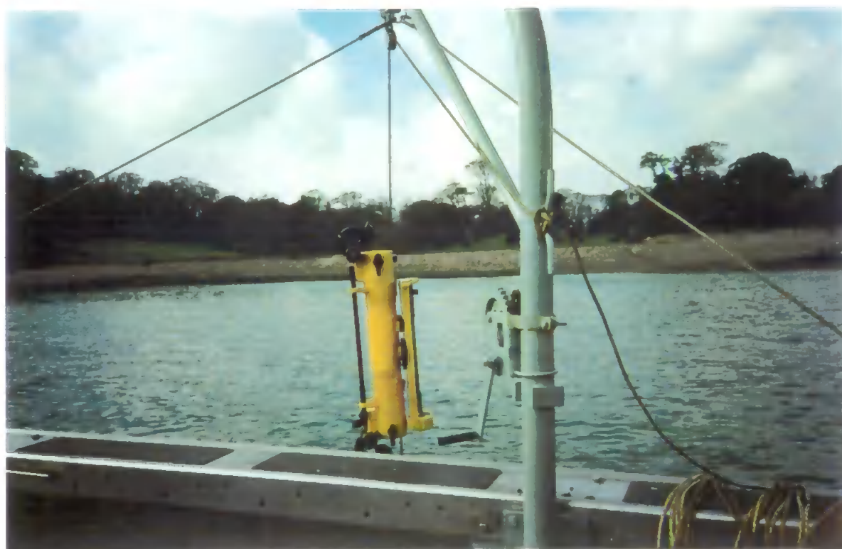
Figure 5.6. Photograph of NIO pattern sampling bottle ready for deployment from the research vessel Tamaris
