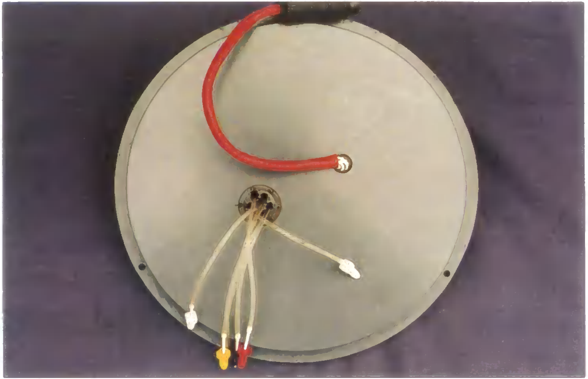
Figure 3.42. View of underside of instrument housing end cap showing detail of internal connections for cable and tubes
