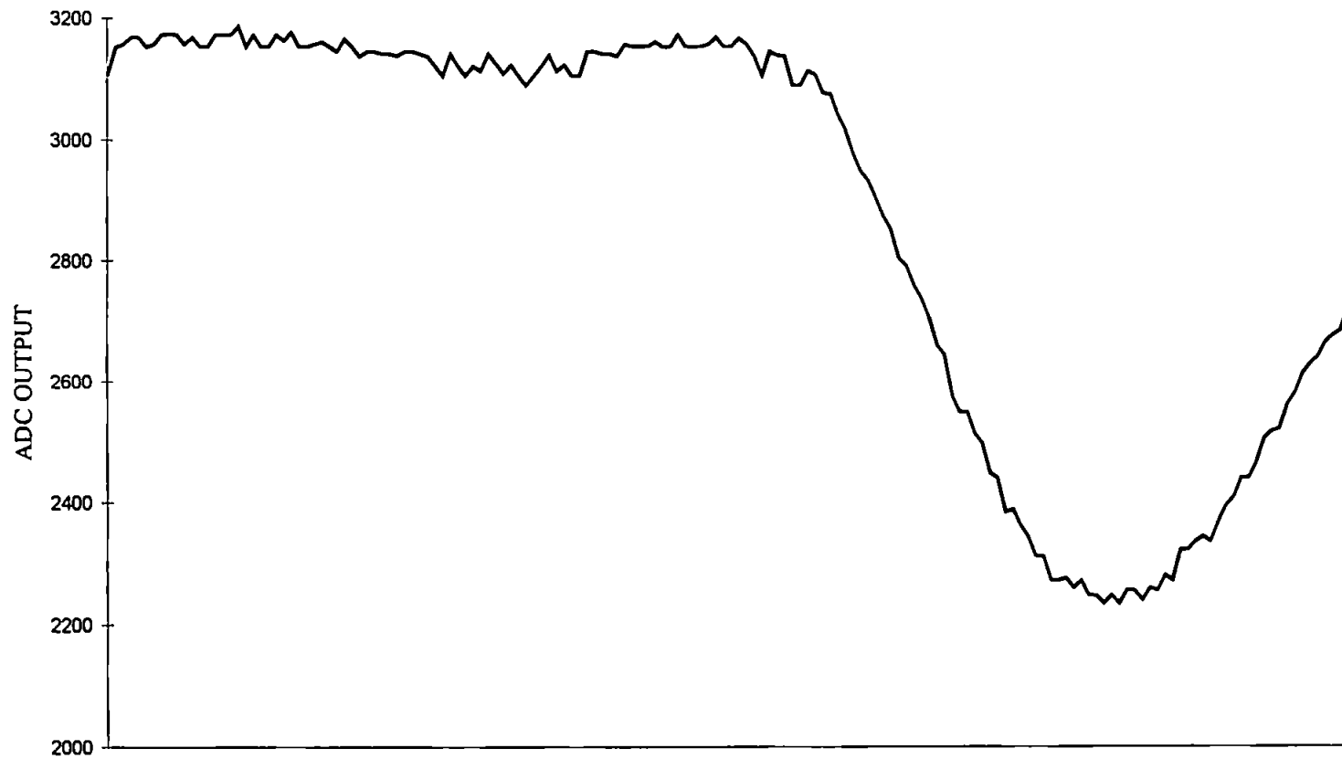
Figure 4.12. Typical peak from the new flowcell with a 5.0 \mu M Nitrite-N standard injection
