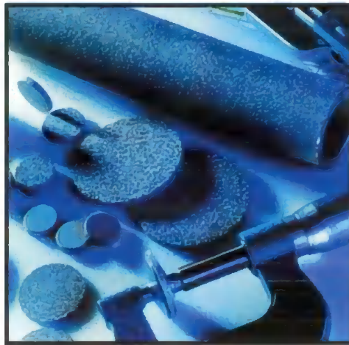
Figure 7.2 Examples of sintered stainless steel media in various moulded configurations.
