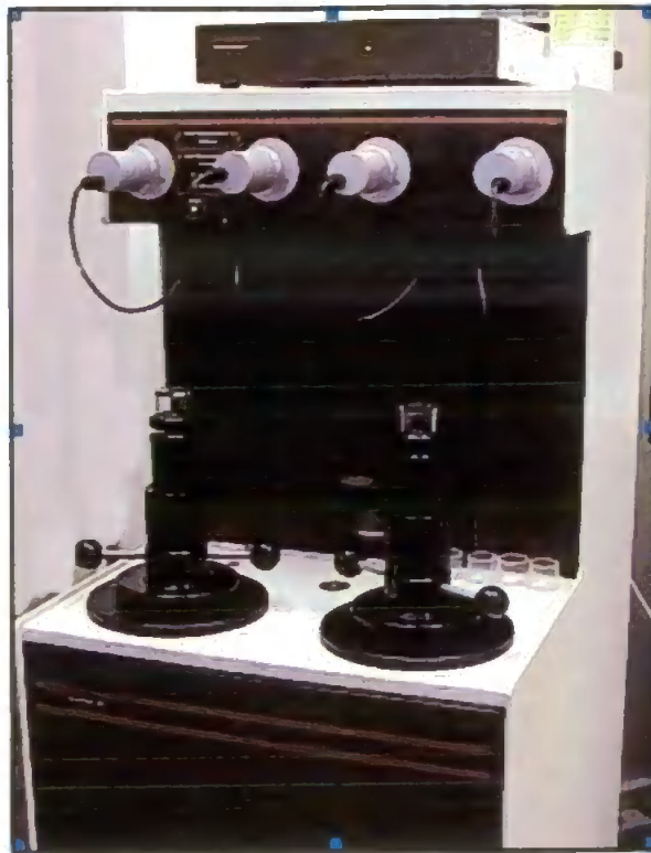
Figure 3.1 Picture of the Auto-Pore III Micromeritics porosimeter showing the four low pressure ports at the top of the instrument (grey cylindrical covers) and the two high pressure oil filled ports (black vertical closure units on the horizontal base).
