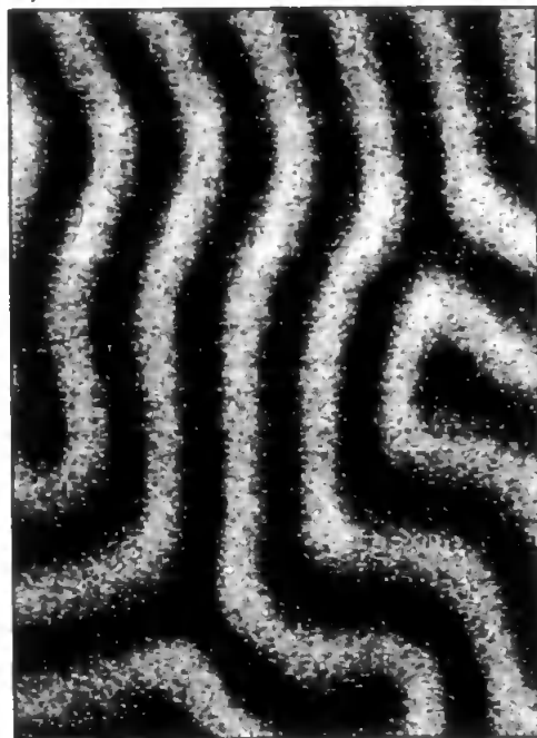
Plate 2 Bubble memory magnetic domain patterns using Kerr effect static laser XY table scan 32\mu\text{m} \times 40\mu\text{m}
