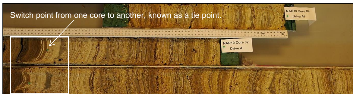
Figure 3.12: Cross-correlations of core sequences from three different core drives.
