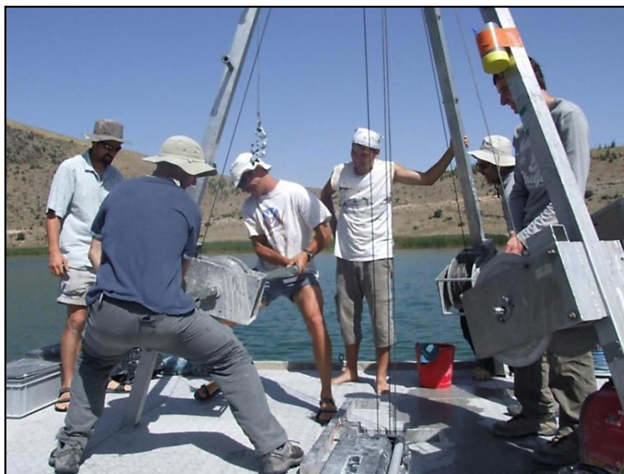
Figure 3.8: UWITEC coring device in operation (extracting the core tubing).
