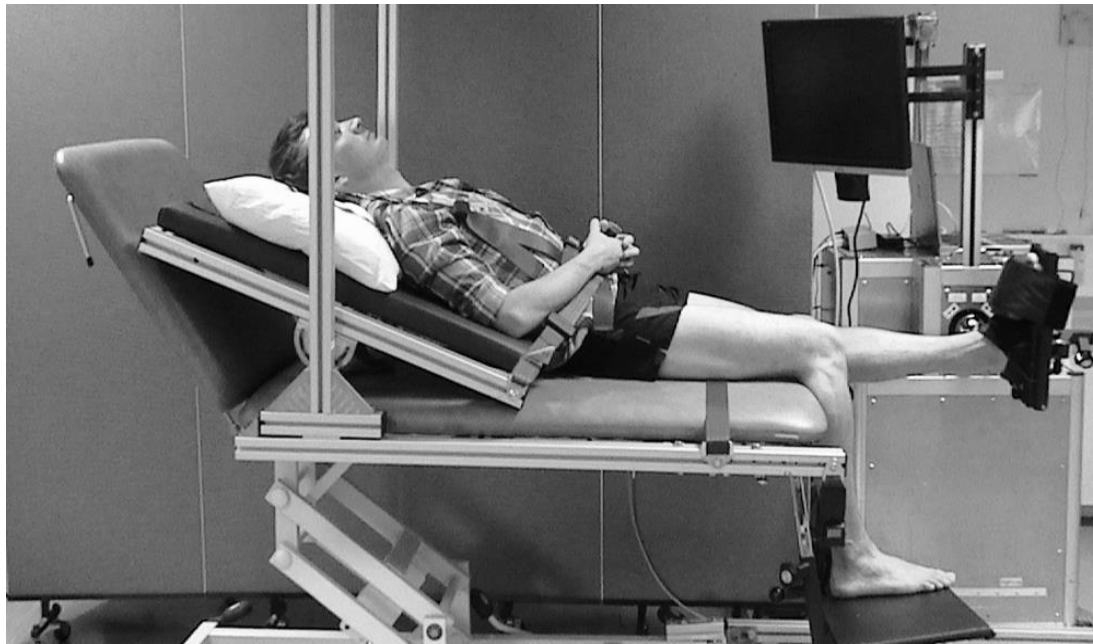
Figure 6.1: Experimental setup: participant in semi-reclined position with the test foot attached to a footplate at 0°.
