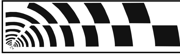
Figure 3.1: Diagram of the LISST-100 ring detector configuration. The shaped photo-detectors are shown by the black areas.
