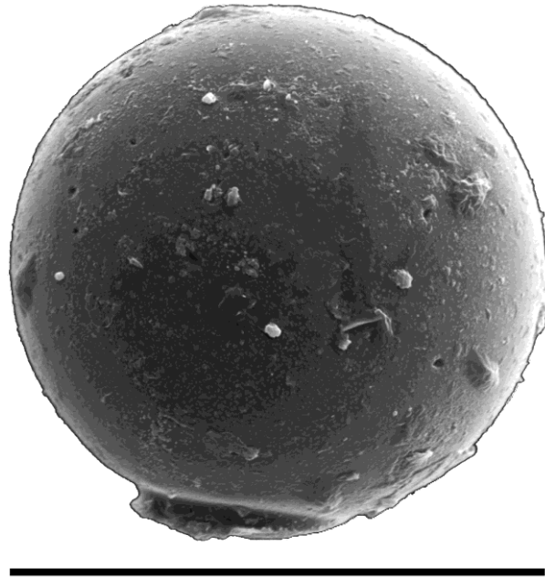
Fig. 12. An example scanning electron microscope image of a Basalt particle used for the data shown in Figure 11. Scale bar is 70 \mu\text{m} .
