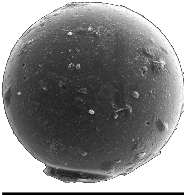
Figure 3.16: An example scanning electron microscope image of a basalt particle used for the data shown in Figure 3.15. Scale bar is 70 \mu m .
