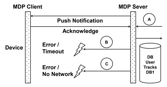
Push Notification: depending on the device or provider, e.g., C2DM (Cloud To Device Messaging, Android), APN (Apple Push Notification), BlackBerry Push Service, Microsoft Push Notification Service, SMS / Flash SMS, ...
