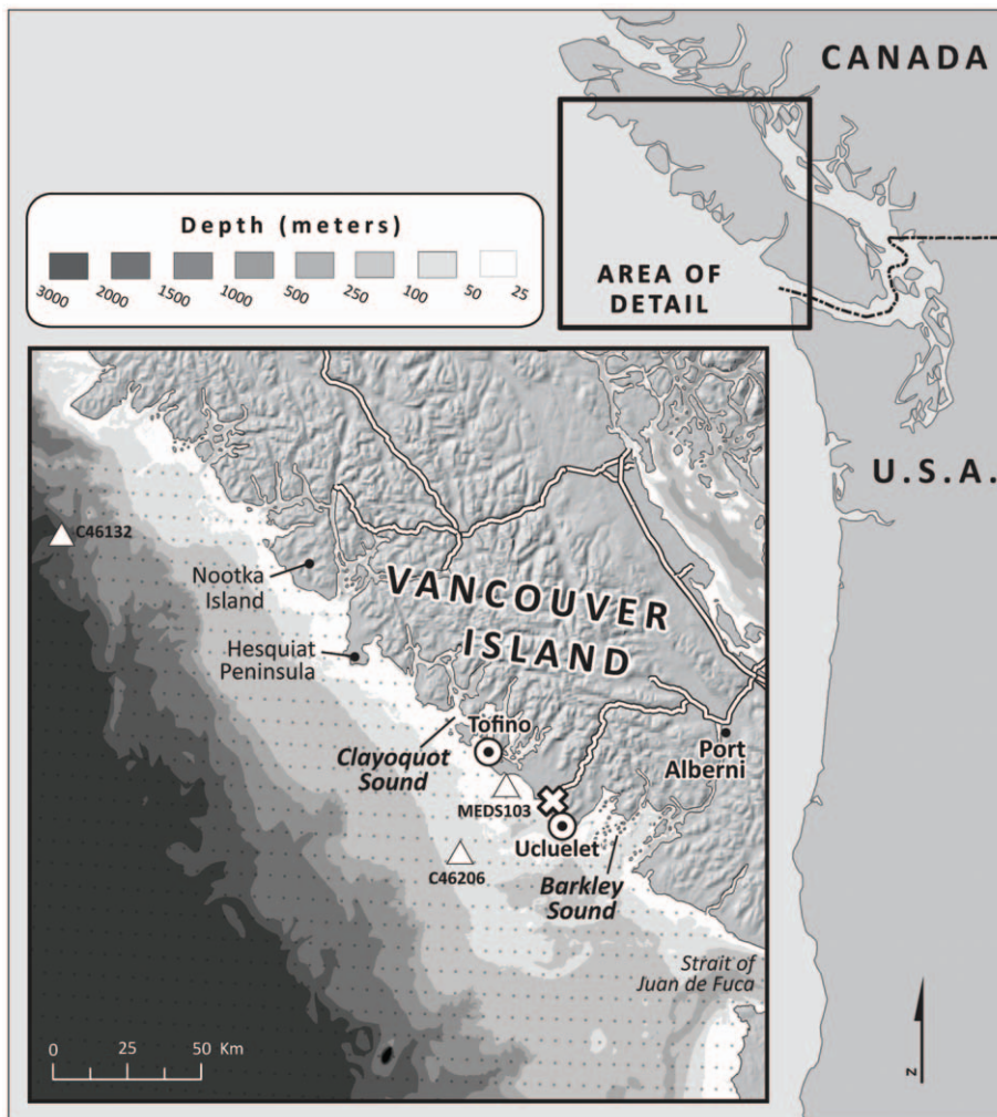
Figure 1. A map of the west coast of Vancouver Island showing three wave buoy stations ( \Delta ), WAVEWATCH III grid points ( \cdot ), and existing transmission lines (black and white line on the Island) connected to Vancouver Island, British Columbia, Canada. Underwater transmission cable landing points ( \odot ) are located in Tofino and Ucluelet. Power grid connection point (empty X) is located in Ucluelet. doi:10.1371/journal.pone.0047598.g001
