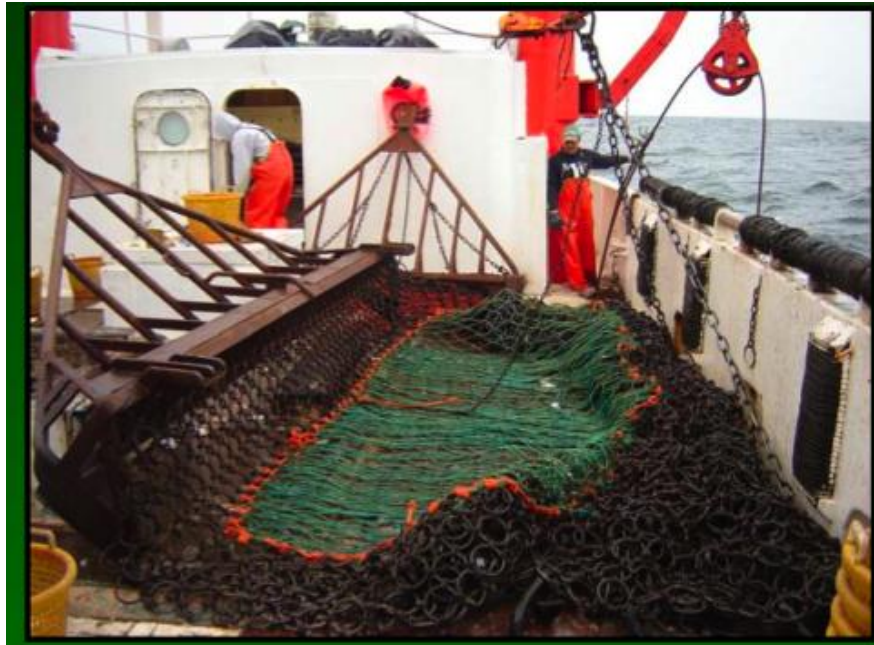
Figure 7: New Bedford sea scallop dredge, showing the steel ring bag and twine mesh panel in the top of the dredge.
