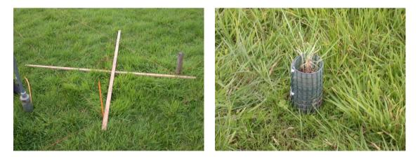
Figure 5C.9 Left: The apparatus used to locate the quadrats centre; the point at which the mesocosm (right) will be placed into the soil.
