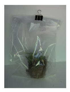
Figure 5A.1 An example of a soil core sealed inside a sunbag to prevent invertebrate contamination whilst maintaining gaseous exchange with the environment.
