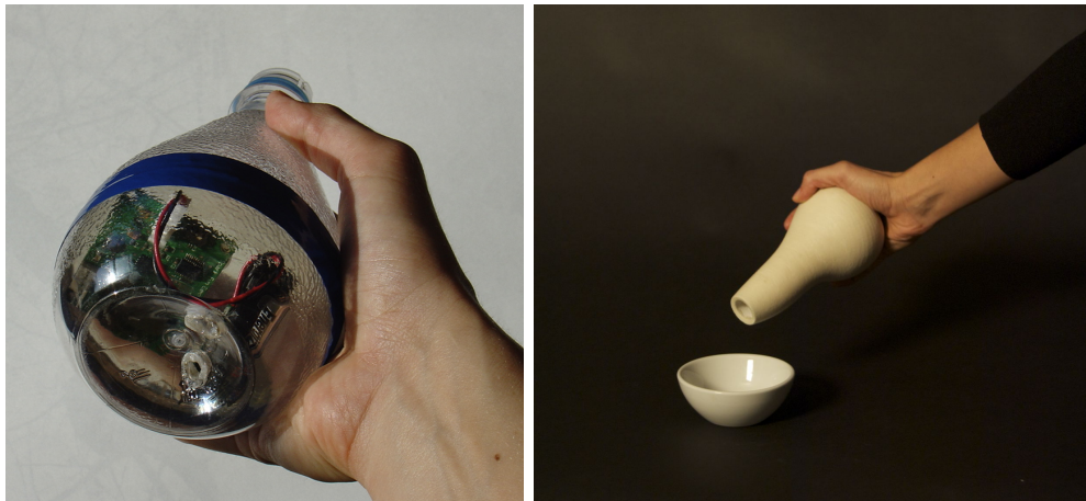
Figure 4.18: The Adaptive Bottle first prototype (left) and final prototype (right) with embedded bluetooth sensors (Franinović and Visell, 2007)
