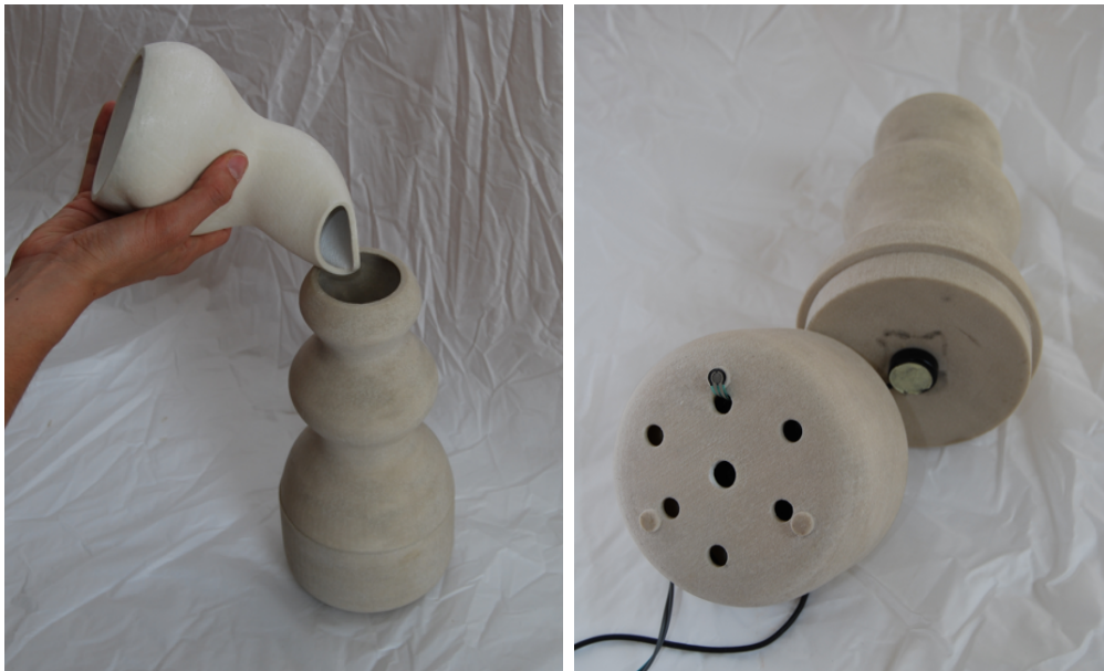
Figure 4.17: The Adaptive Bottle : the receptacle and the bottom part hosting speaker and sensing system. (Franinović and Visell, 2007)
