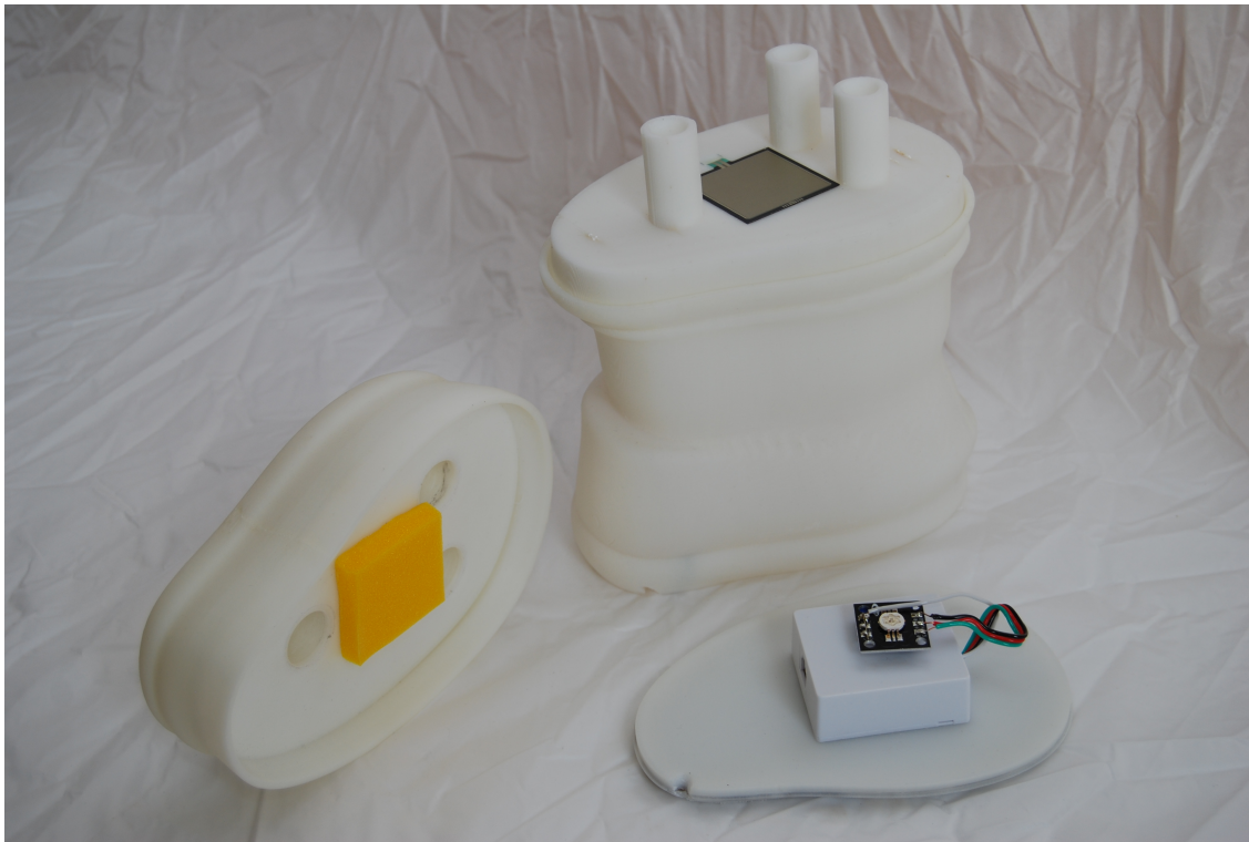
Figure 4.16: The Crushhh prototype with force-sensitive resistor and LED module (Franinović and Visell, 2007)
