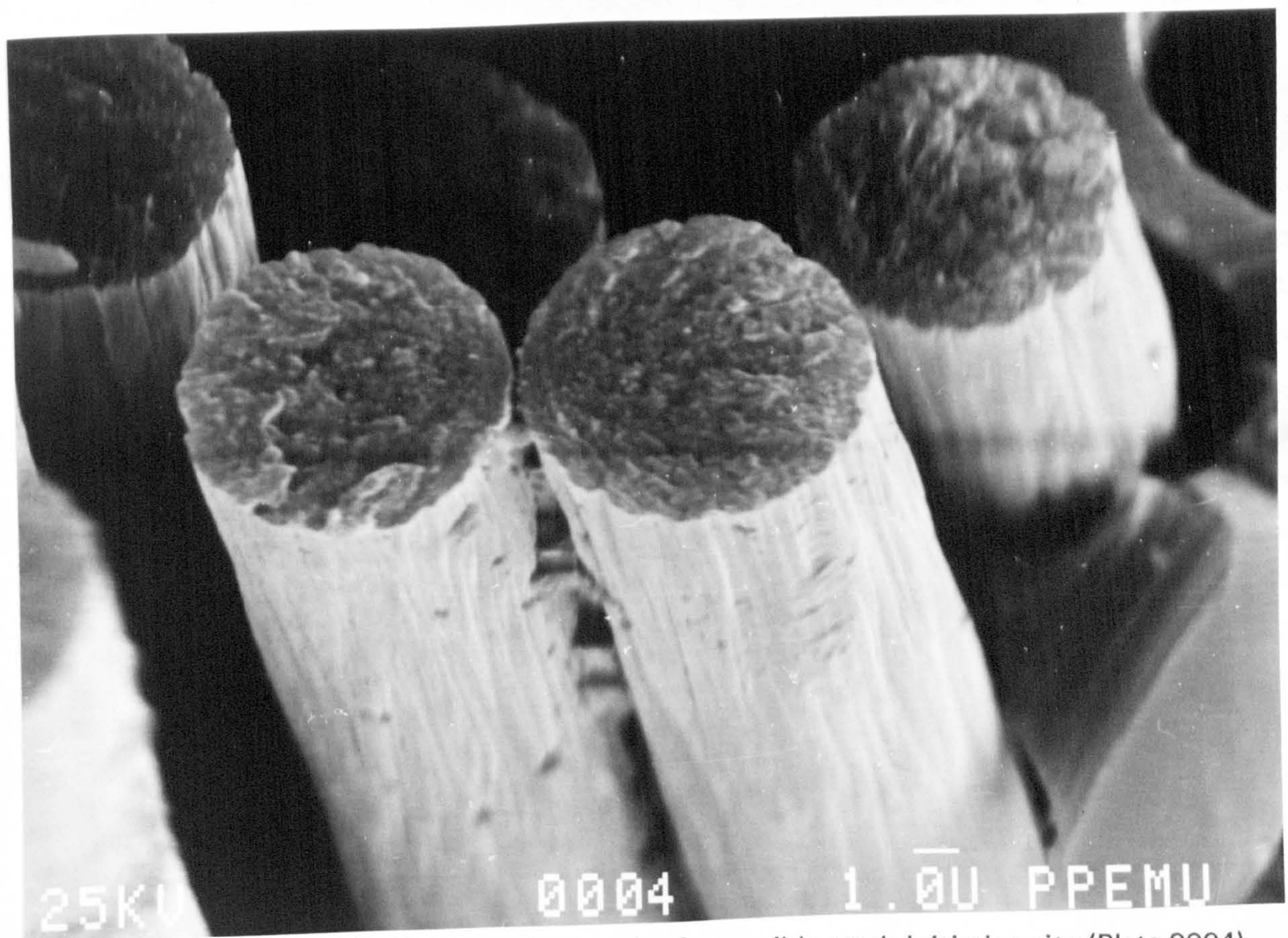
Figure 43: Electron micrograph of a cluster of carbon fibres in plate 0008 (Plate 0009)
