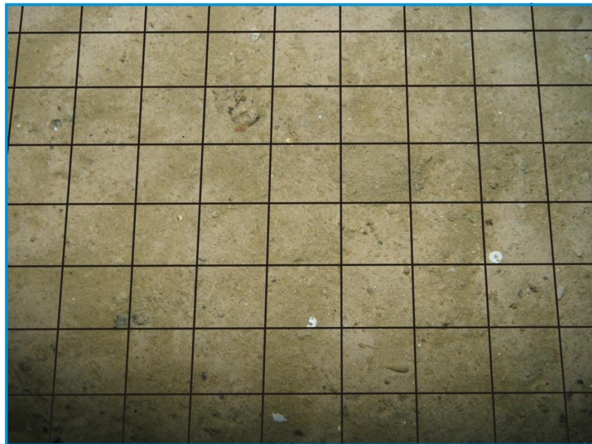
Fig. 2.5: Image of the calibration grid (on bottom) overlaid on a sample image from the 2009 survey. The grid cell size is 4.9 cm (vertical in figure) by 5.5 cm (horizontal in figure).
