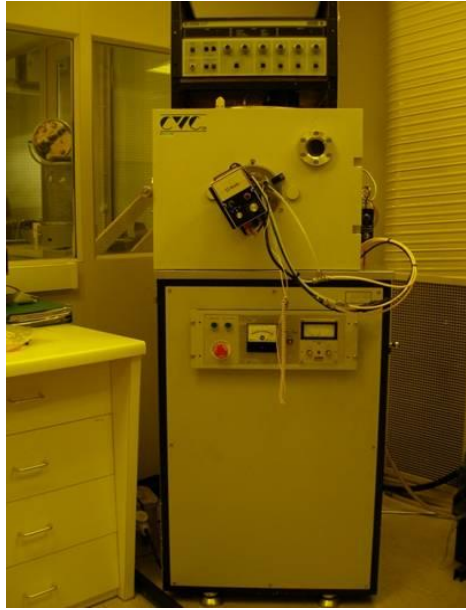
Fig. 3.9. Picture of the ion miller used for the work.
