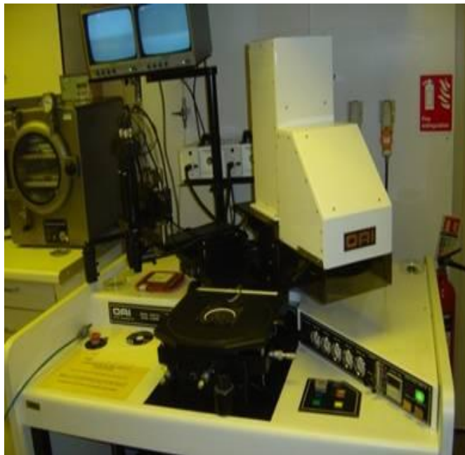
Fig. 3.8. Picture of the OAI 500 mask aligner used for the work.
