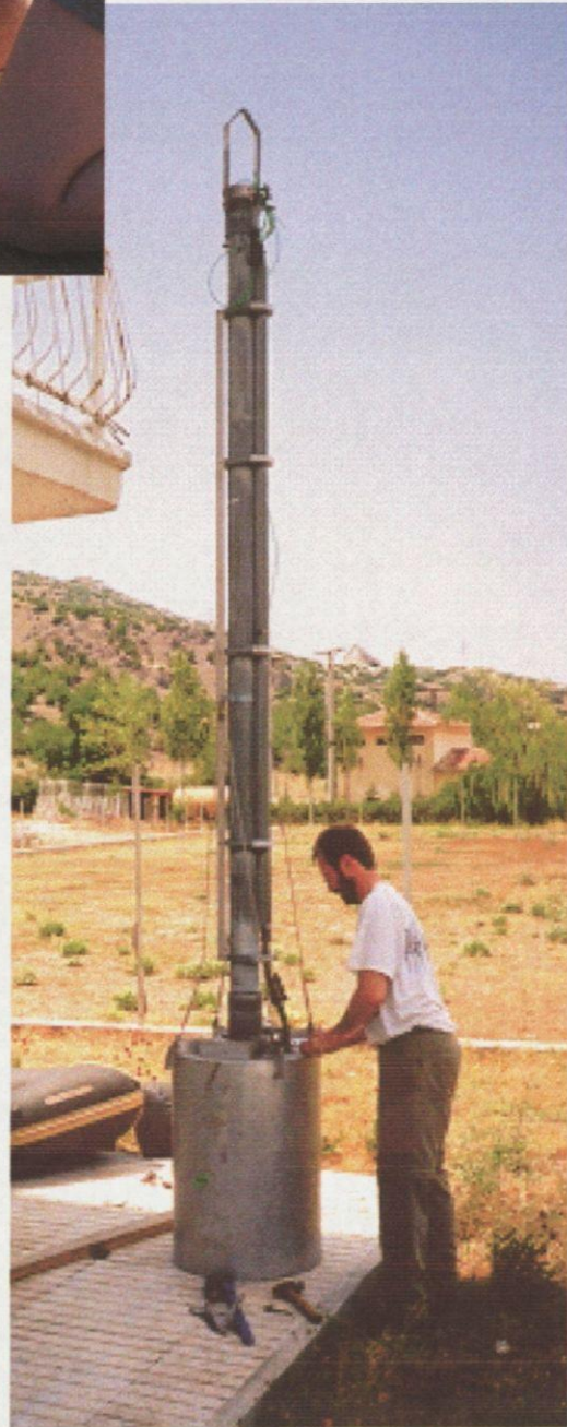
Fig. 4.3 The 3m Mackereth corer.
