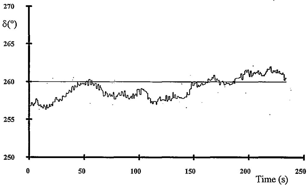
Figure 7.13 Heading Response for SOC Autopilot (Learning On) During Course-Keeping with a Desired Heading of 260°
